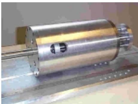
*Fig. 1: The multi-airgap linear actuator prototype*
