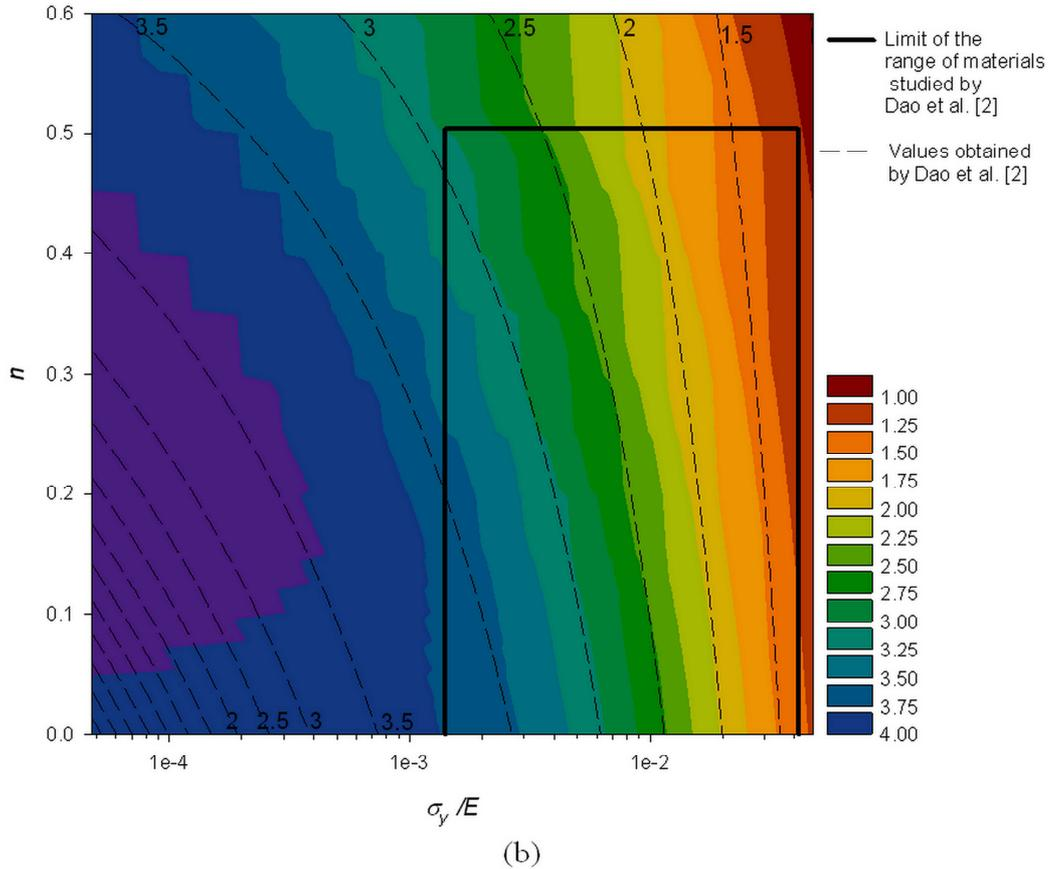
Fig. 12: Values of the  $HM/\sigma_R$  ratio obtained from Eqs. (2) and (3) and the values of representative strain. (a): comparison with the values of Dao et al. (2001); (b): comparison with the values of Cao and Huber (2006).
