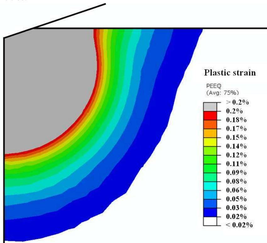
Fig 13: Plastic strain distribution induced by conical indenter equivalent to the Vickers indenter obtained for a material with  $E=120000$  MPa,  $\sigma_Y= 3$  MPa and  $n=0.466$  (material similar to that studied by Prasad et al. (2011)).
