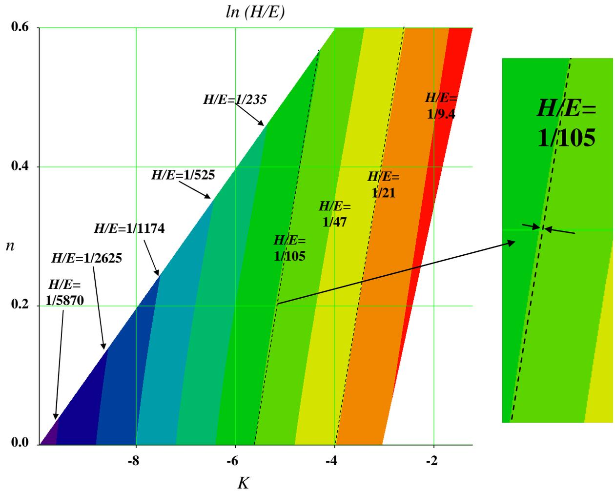
Fig. 3:  $H/E$  ratio values obtained for the various values of  $n$  and  $K$  parameters studied in this work.
