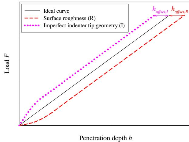
**Fig.1.** Effect of low scale artefacts on the indentation curve
