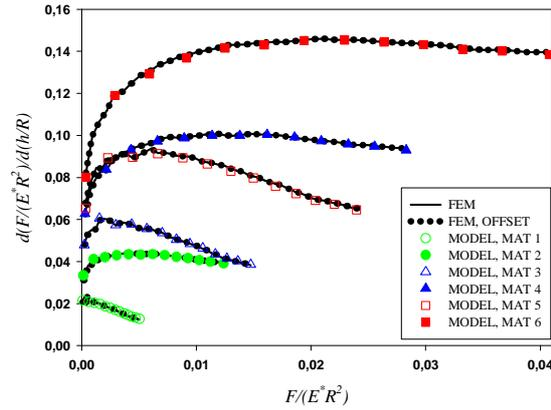
**Fig.7.** Slope of the indentation curve versus indentation load for the indentation curves obtained from the FEM simulations, non offset and offset, and for the indentation curves obtained from the model
