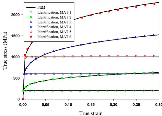
**Fig.8.** Comparison of the stress-strain identified from offset FEM indentation curves to the stress-strain curves used in the FEM simulations, minimising  $\omega_2$
