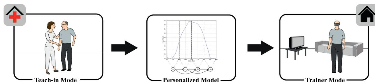
Fig. 3. Overview of the personalized exercise trainer use case. During the guided *Teach-in Mode* a reference motion is recorded. Based on the captured motion data a *Personalized Model* is generated. In the *Trainer Mode* at home the model is used as personal evaluation reference. An individual model is trained for each exercise.
