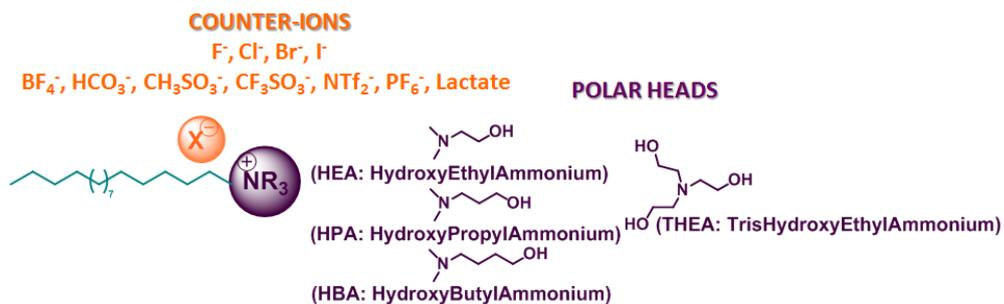
**Figure 2.** *N*-(hydroxyalkyl)cetylammonium salts as efficient protective agents of size- and morphology-controlled Rh<sup>0</sup> NPs
