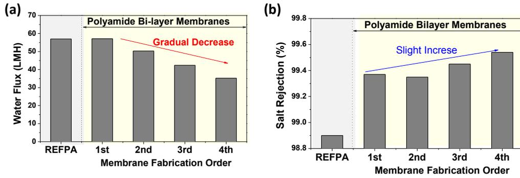
**Figure 2.** Water flux (a) and salt rejection (b) of REFPA and four coupons of polyamide bilayer membranes (1<sup>st</sup> ~ 4<sup>th</sup>) prepared by sequential interfacial polymerization in the manner of serial membrane dipping.
