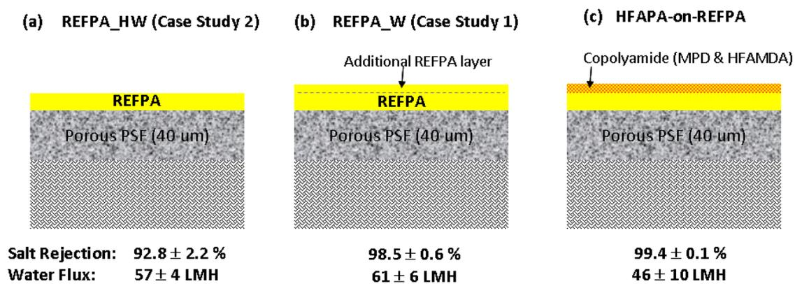
**Figure 5.** Expected structures of RO membranes made by three different processes and their desalination performance (a) REFPA made by the process shown in the case study 2 (w/additional hexane rinse), (b) REFPA made by the process shown in the case study 1, and (c) polyamide bilayer membrane made by the SIP process shown in Figure 1.
