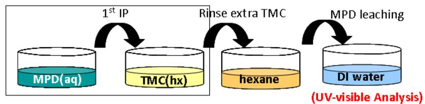
**Figure 3.** Schemes for the case studies to prove MPD leaching and its reactivity in the 2<sup>nd</sup> aqueous solution
