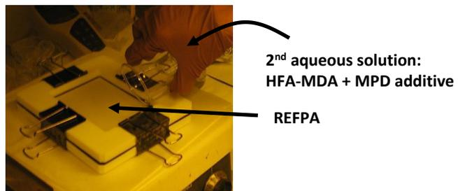
**Figure 6.** A photograph showing a frame process to form polyamide bilayer membranes featuring HFAPA top-layer (copolymerization of HFAMDA and MPD additive) on a REFPA under-layer without cross-contamination
