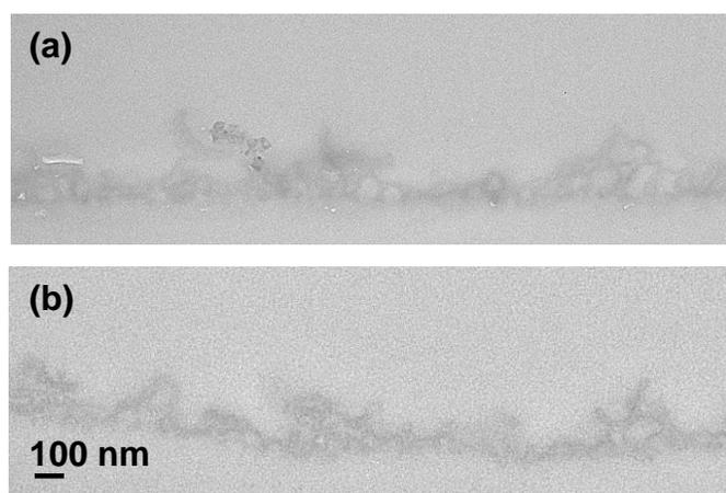
**Figure S1.** Cross-sectional TEM images of (a) REFPA and (b) HFAPA-on-REFPA membranes. The first sample coupon of HFAPA-on-REFPA was used for TEM analysis.
