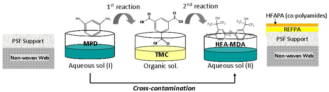
**Figure 1.** A schematic drawing showing a cross-contamination issue in the sequential interfacial polymerization (SIP) process based on the subsequent membrane dipping.
