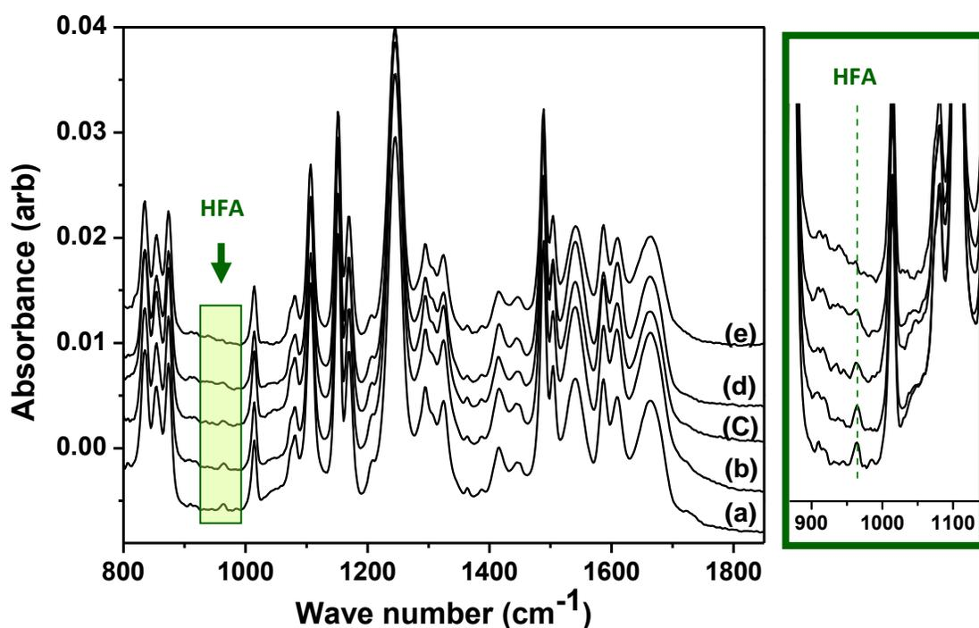
**Figure 7:** FTIR spectra of polyamide bilayer membranes prepared by adding various amount of MPD additive into the 2nd aqueous solution containing HFA-MDA monomer ((a) 0 %, (b) 1.2 %, (c) 2.4 %, (d) 4.8 %, and (e) 100 % MPD additions). (a), (b) ~ (d), and (e) spectra were originated from a pure HFAPA top-layer, copolyamide top-layers, and a pure REFPA top-layer on REFPA under-layers, respectively. Green box on the right: magnified spectra in the range of 900 ~ 1100 cm<sup>-1</sup>.
