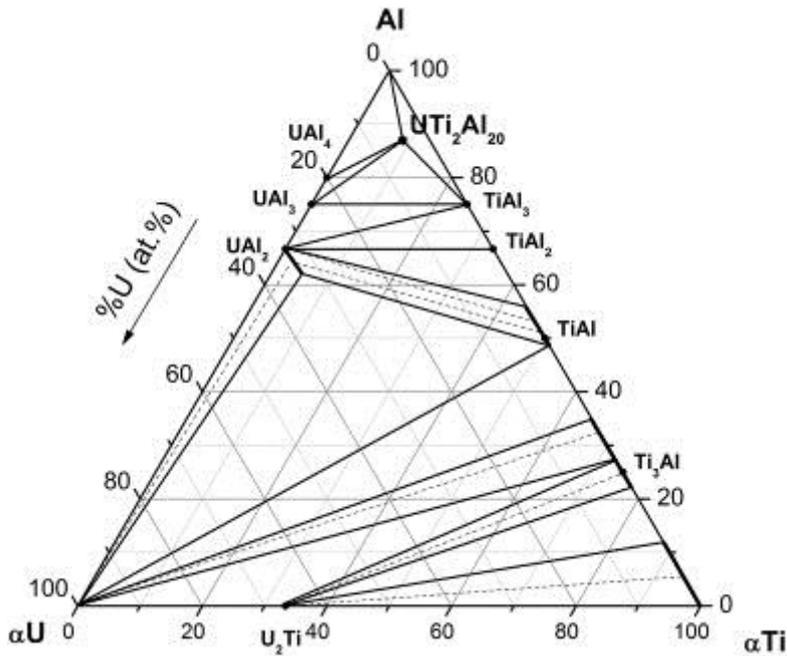
**Figure.1:** Phase relations in the ternary U-Ti-Al system, constructed from samples heat-treated at 923K
