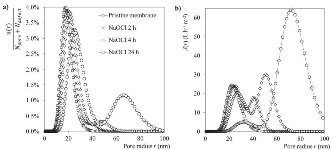
**Figure 10:** a)  $n(r)$  the discontinuous distribution of the number of pores and of defects and b)  $J(r)$  the flow density relative to each pore size class for pristine and aged membrane samples according to the second scenario
