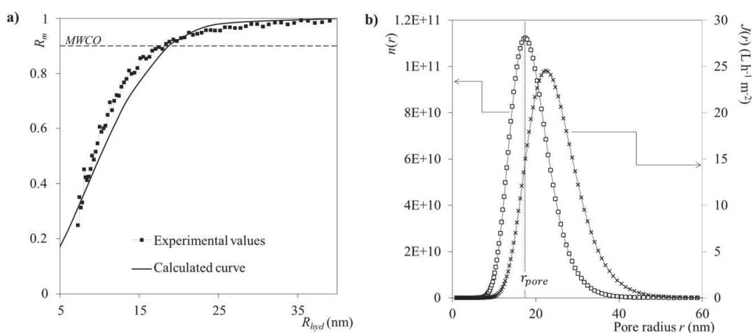
Figure 7: (a) Calculated and experimental selectivity curves for pristine membrane and (b)  $n(r)$  the discontinuous distribution of the number of pores and  $J(r)$  the flow density relative to each pore size class
