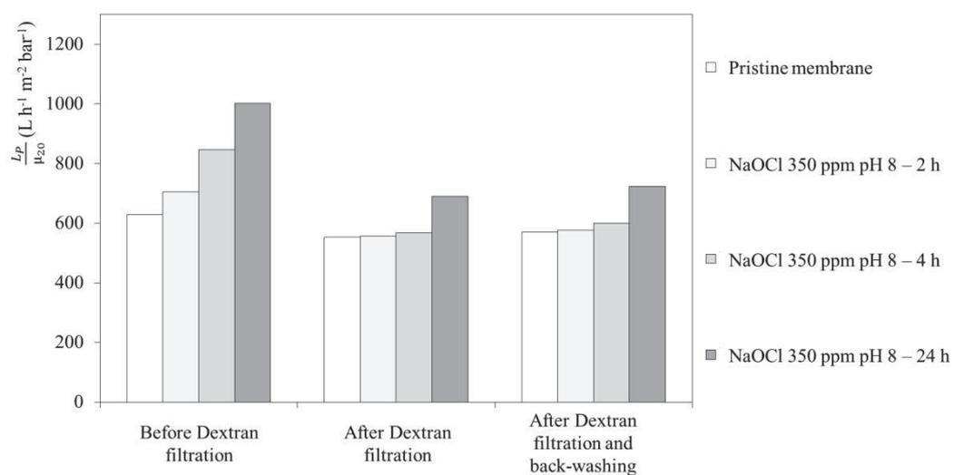
**Figure 5:** pure water permeability of pristine and aged membrane samples, before and after Dextran filtration test and after back-washing with ultrapure water
