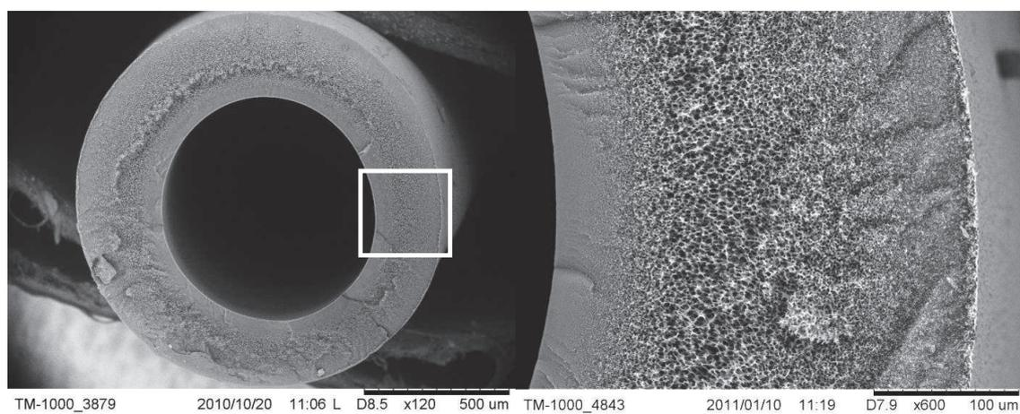
Figure 1: Cross-section SEM image of a cryo-fractured pristine membrane
