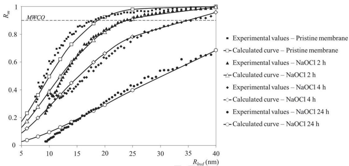
**Figure 9:** Selectivity curves of pristine and aged membranes (*NaOCl* 350 ppm, pH 8), comparison between experimental results and calculated ones according to the second scenario.
