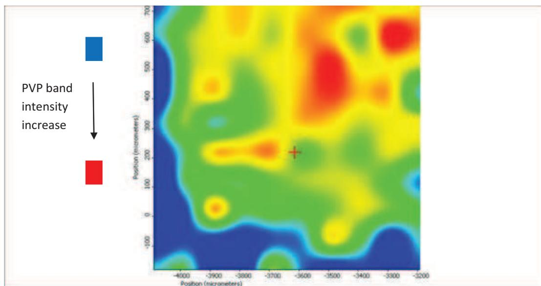
**Figure 11:** 2D mapping by ATR - IRTF of the inner surface of pristine membrane showing the amide band intensity of PVP (from Prulho [29])
