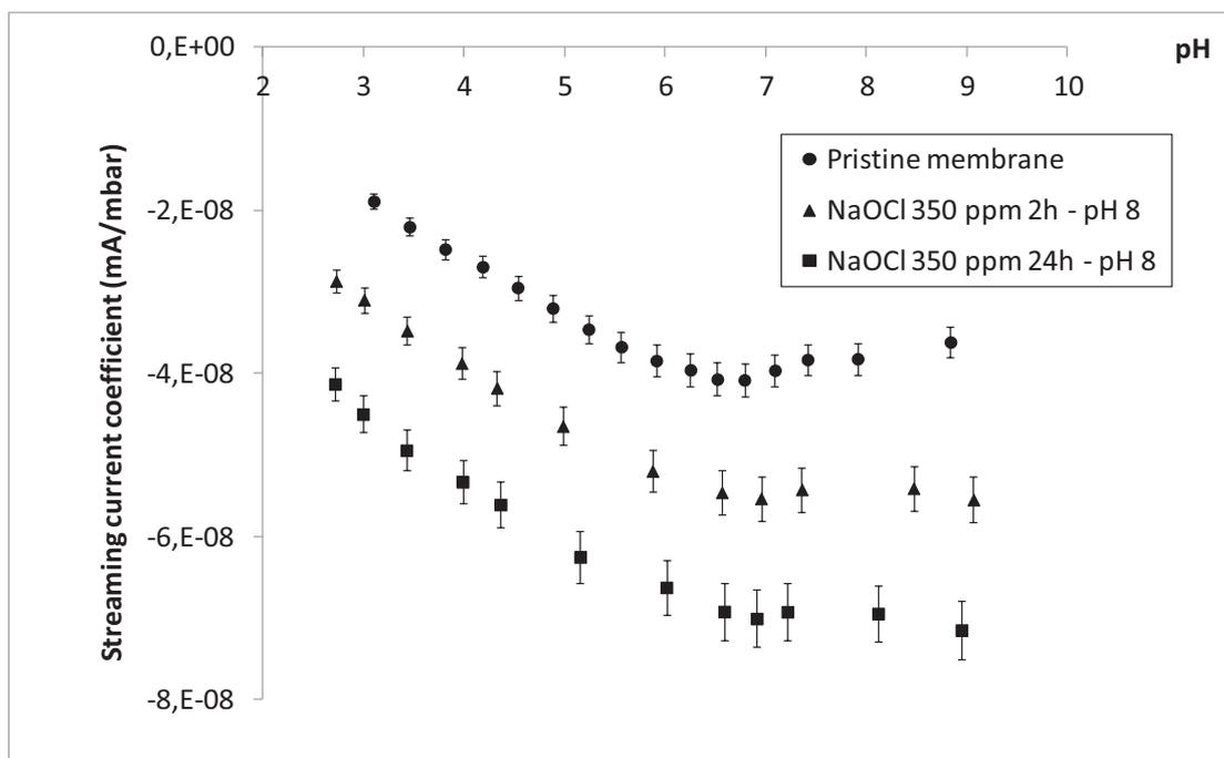
Figure 3: Streaming current coefficient ( $I_s / \Delta P$ ) of pristine and aged membranes as a function of pH.
