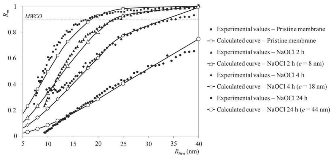
**Figure 8** Selectivity curves of pristine and aged membranes (*NaOCl* 350 ppm, pH 8), comparison between experimental results and calculated ones using a pore size distribution in which ageing induced an increase in pore radius (first scenario).
