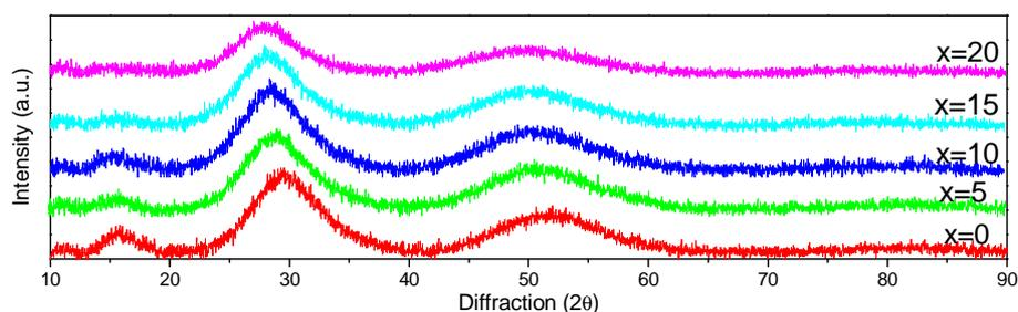
Fig. 2. XRD pattern of the  $\text{Ge}_{20}\text{Sb}_5\text{Se}_{75-x}\text{I}_x$  glass samples
