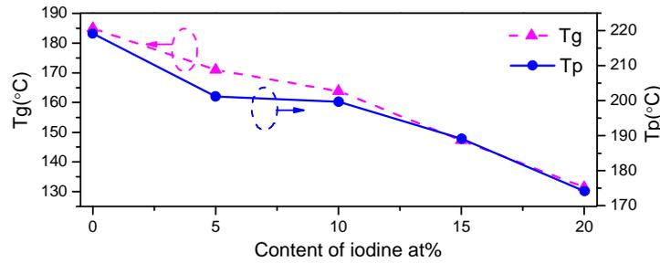
Fig. 4. Thermal parameters of the  $\text{Ge}_{20}\text{Sb}_5\text{Se}_{75-x}\text{I}_x$  glass samples
