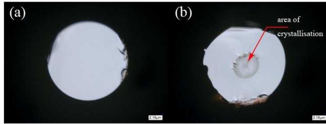
Fig. 10. Drawn fiber end under the digital microscope:
