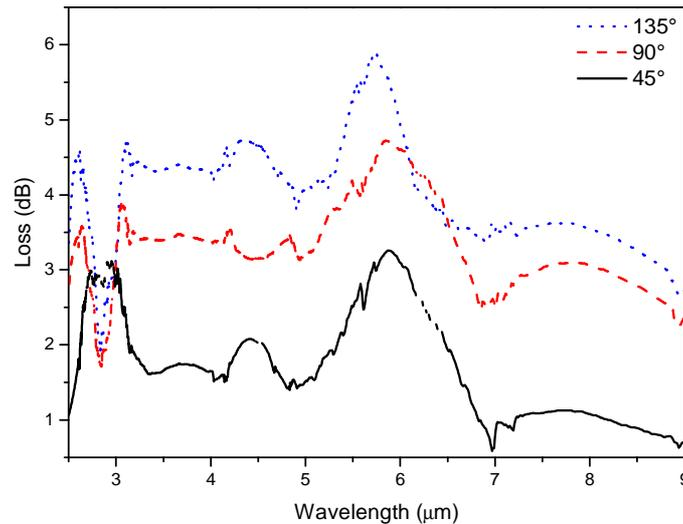
Fig. 12. Bend loss spectra of the Ge<sub>20</sub>Sb<sub>5</sub>Se<sub>55</sub>I<sub>20</sub> optical fiber
