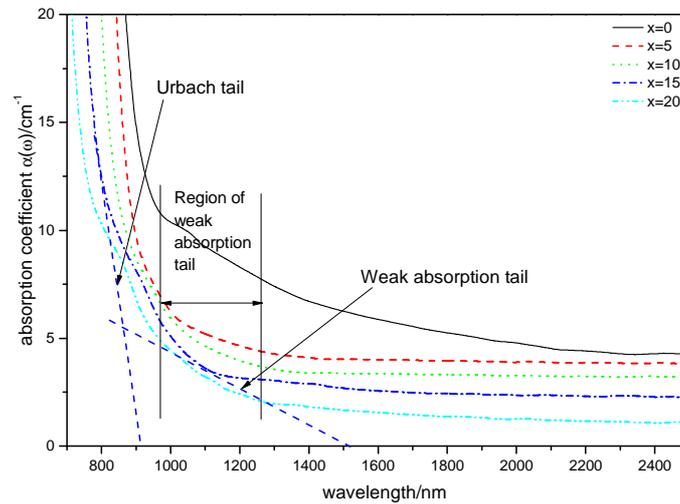
Fig. 5. Absorption spectra of the  $\text{Ge}_{20}\text{Sb}_5\text{Se}_{75-x}\text{I}_x$  glass samples.
