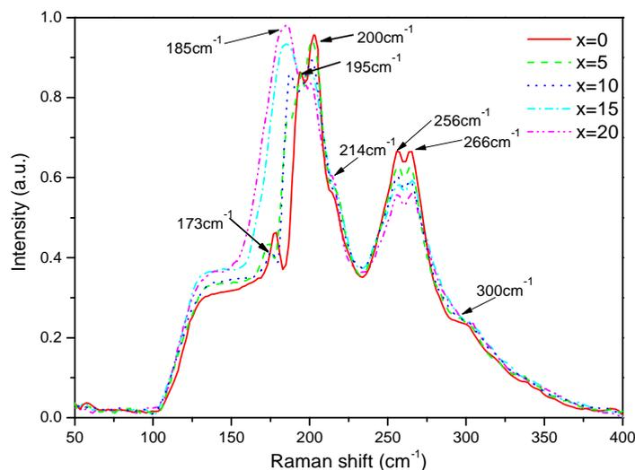
Fig. 7. Normalized Raman spectra of the  $\text{Ge}_{20}\text{Sb}_5\text{Se}_{75-x}\text{I}_x$  glasses
