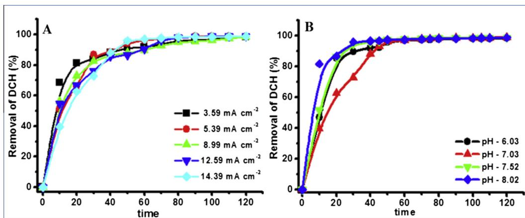
**Figure 3** Removal of DCH as a function of current density (A) and pH of the solution (B). Conditions: (A) pH = 7, [DCH] = 100 mg L<sup>-1</sup>, Q = 52 L min<sup>-1</sup>, d = 1 cm, conductivity = 1.78 mS cm<sup>-2</sup>; (B) [DCH] = 100 mg L<sup>-1</sup>, CD = 5.39 mA cm<sup>-2</sup>, Q = 52 mL min<sup>-1</sup>, d = 1 cm, conductivity = 1.78 mS cm<sup>-1</sup>.
