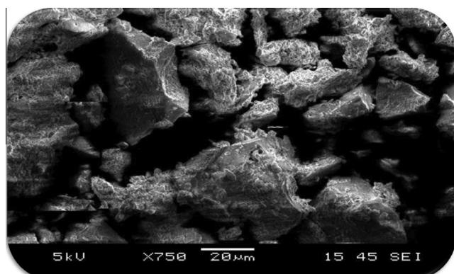
**Figure 8** Scanning electron micrographs of electro-generated aluminum coagulant.
