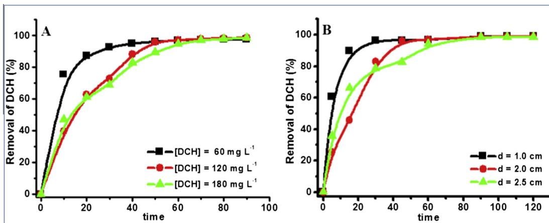
**Figure 4** Removal of DCH as a function of initial DCH concentration (A) and spacing between electrodes (B). Conditions: (A) pH = 7, CD = 5.39 mA cm<sup>-2</sup>, Q = 52 mL min<sup>-1</sup>, d = 1 cm, conductivity = 1.78 mS cm<sup>-1</sup>; (B) pH = 7, [DCH] = 100 mg L<sup>-1</sup>, CD = 5.39 mA cm<sup>-2</sup>, Q = 52 mL min<sup>-1</sup>, conductivity = 1.78 mS cm<sup>-1</sup>.
