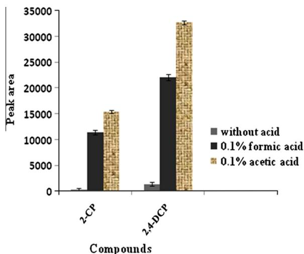
**Figure 1** Influence of the presence of acetic acid and formic acid in mobile phase (acetonitrile/ultrapure water (55:45, v/v)) on the chlorophenols measured responses. The mobile phase was modified with 0.1% formic acid and 0.1% acetic acid in water.
