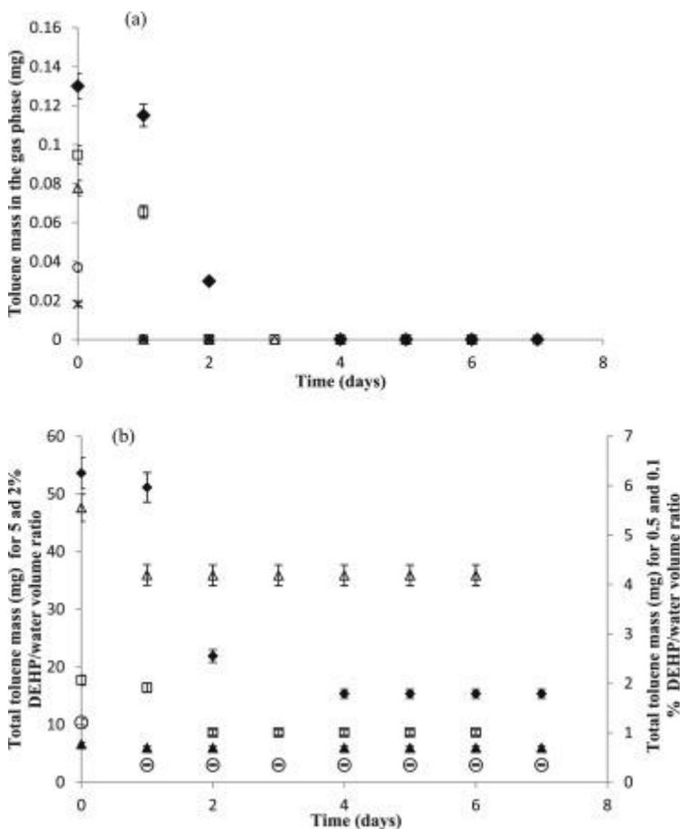
**Figure.2.** Time-course of toluene amount in the gas phase (a) and its total amount (b) during biodegradation by activated sludge in batch culture for an initial toluene concentration in DEHP of 4.3 g/L, pH =7, T=25°C, stirring rate = 300 rpm.
