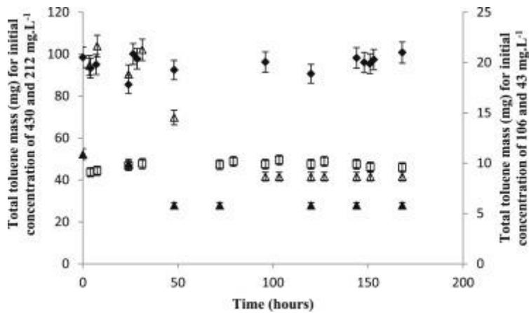
**Figure.4.** Time-course of toluene total amount during biodegradation by activated sludge in batch culture for a volume ratio DEHP in water of 0.1 %, pH =7, T=25°C, stirring rate = 300 rpm. ◆ 430 mg l<sup>-1</sup> □ 212 mg l<sup>-1</sup> △ 106 mg l<sup>-1</sup> ▲ 43 mg l<sup>-1</sup>
