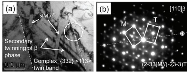
Fig. 3. TEM characterization of the deformation twinning in the deformed alloys ( $\epsilon=0.05$ ). (a) Bright-field image of a mechanical twin; (b) the corresponding selected area electron diffraction (SAED) pattern on the twinning interface identifies a  $(2-33)[31-1]$  twinning relationship.
