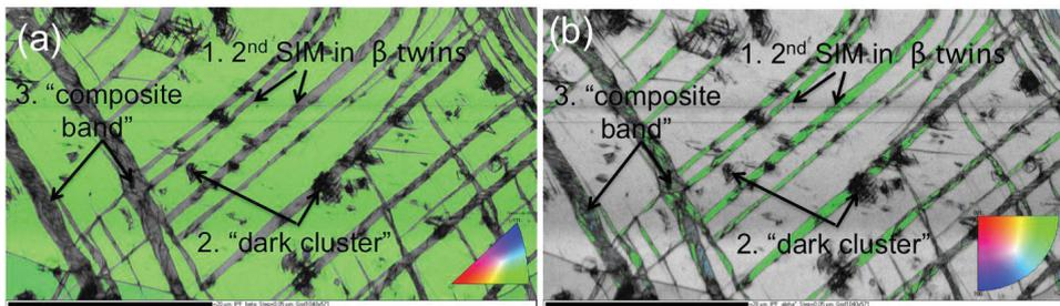
Fig. 4. EBSD orientation contrast imaging of the deformed alloy ( $\epsilon=0.05$ ). (a) orientation map of  $\beta$  phase; (b) orientation map of SIM  $\alpha''$  precipitates. Three microstructural features are shown in the figure: 2<sup>nd</sup> SIM  $\alpha''$  in  $\beta$  twins, the “dark clusters” and “composite band”, numbered by 1, 2 and 3, respectively.
