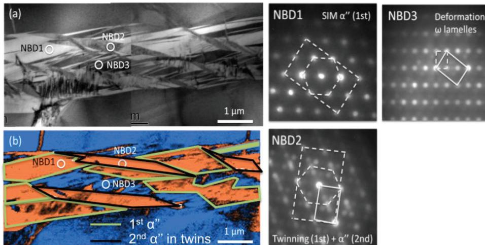
Fig. 6. TEM characterizations on the feature “composition band”, (a) TEM bright-field image of the “composite band”; (b) ACOM-TEM phase mapping of SIM  $\alpha''$  (orange) and  $\beta$  phase (blue). The key NBD patterns of each zone of interest are also given. A schematic drawing of the different phase blocks are added onto the (b) ACOM-TEM mapping [25].
