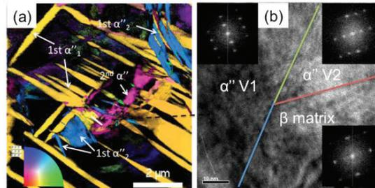
Fig. 5. TEM characterizations on the feature “dark clusters”, (a) ACOM-TEM orientation mapping of SIM  $\alpha''$  variants; (b) HRTEM imaging of a joint position among two  $\alpha''$  variants and  $\beta$  matrix.
