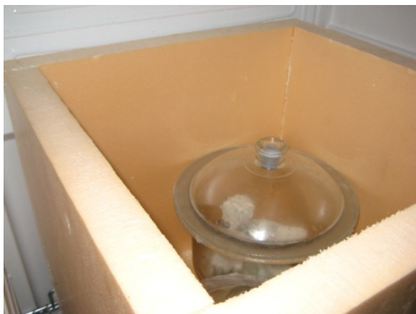
Fig. 2 Desiccators in the insulating box
