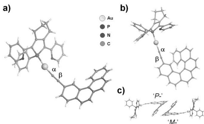
**Figure 2.** Views of the X-ray structures of (a) **1a** (only one of the two symmetrically independent molecules found in the unit cell of **1a** is shown); (b) *rac-1b* (only *M*-(+)-stereoisomer is shown) and (c) heterochiral  $\pi$ -dimers observed in the centrosymmetric crystal of *rac-1b*.
