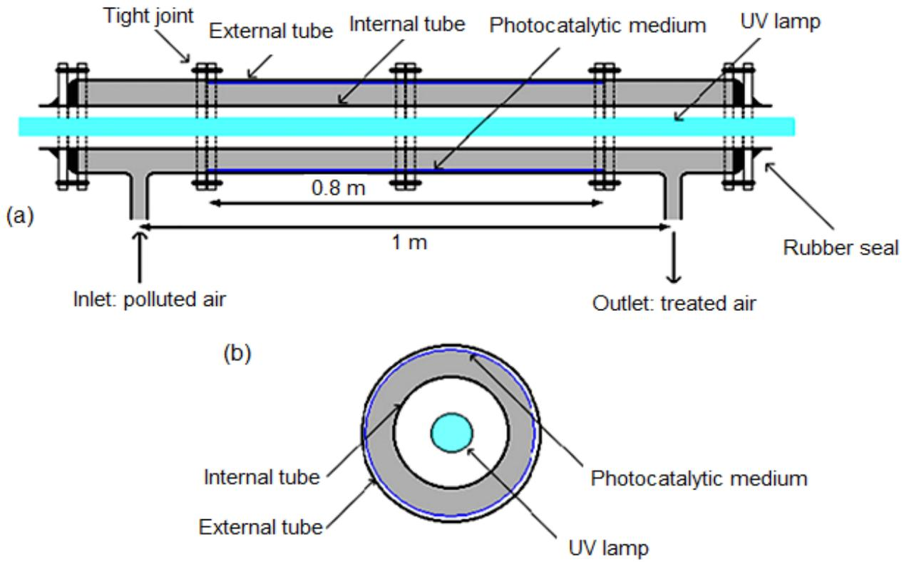
Fig. 1: Scheme (a) and sectional drawing (b) of the cylindrical photoreactor
