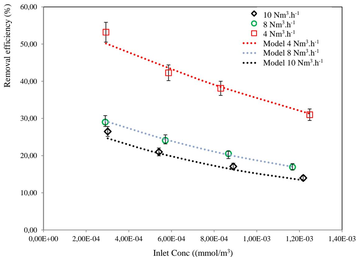
Fig. 8: Variation of removal efficiency of isovaleraldehyde with the inlet concentration at different flowrates in planar reactor (Air gap= 20 mm, T = 20°C, RH = 50 %, I = 24Wm<sup>-2</sup>).
