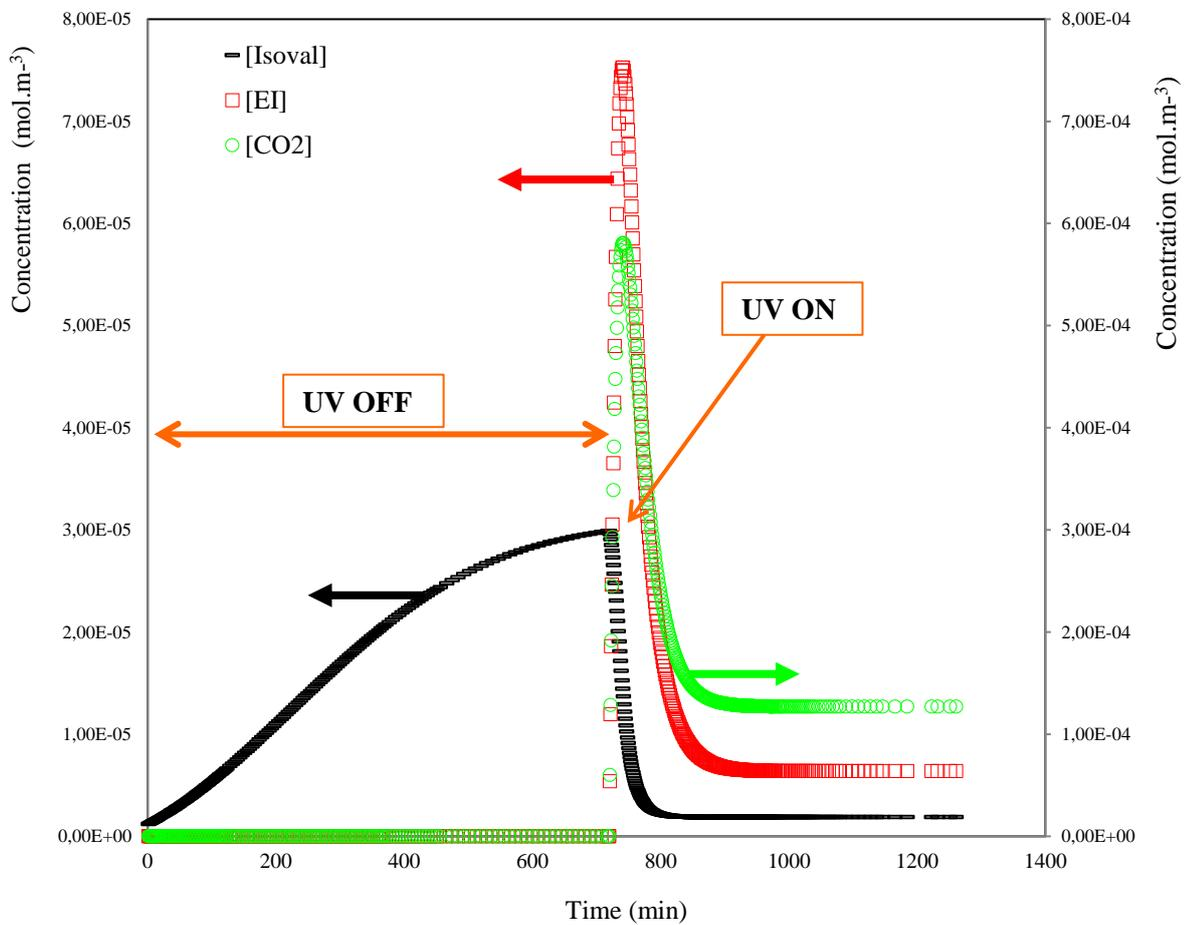
Fig.6: Computed concentration of isovaleraldehyde and byproducts versus simulation time
