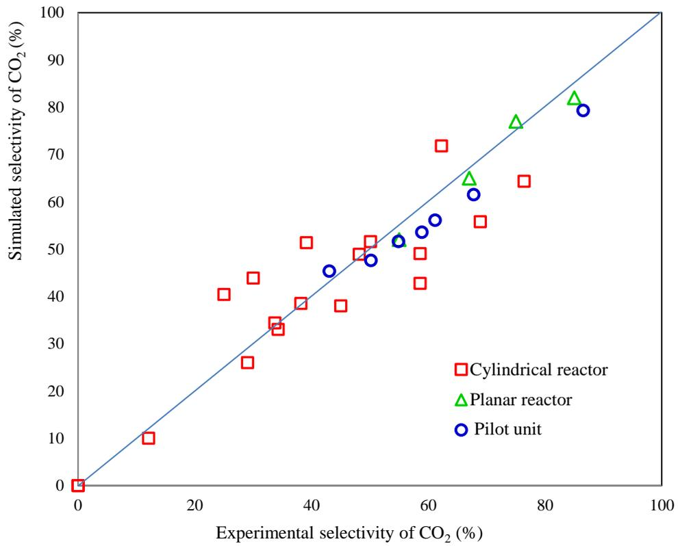
Fig. 10: Comparison of simulated results of CO<sub>2</sub>'s selectivity vs. experimental data at different flowrates and inlet concentrations using three reactors.
