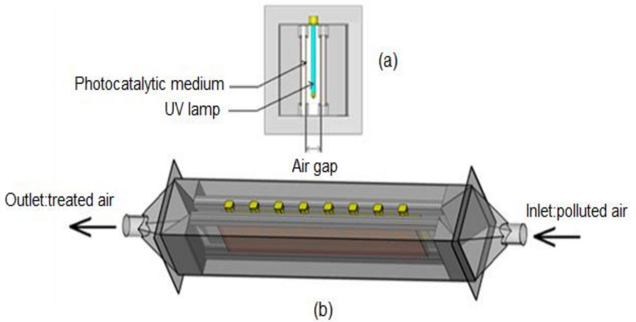
Fig.2: Scheme (b) and sectional drawing (a) of the planar photoreactor
