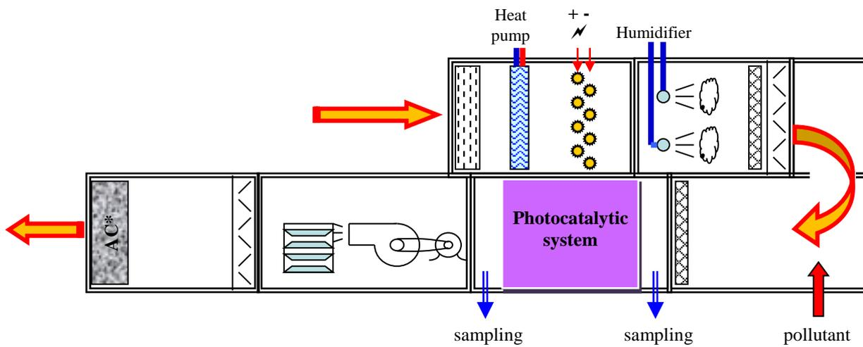
Fig.3: A functional diagram of pilot unit (CIAT)
