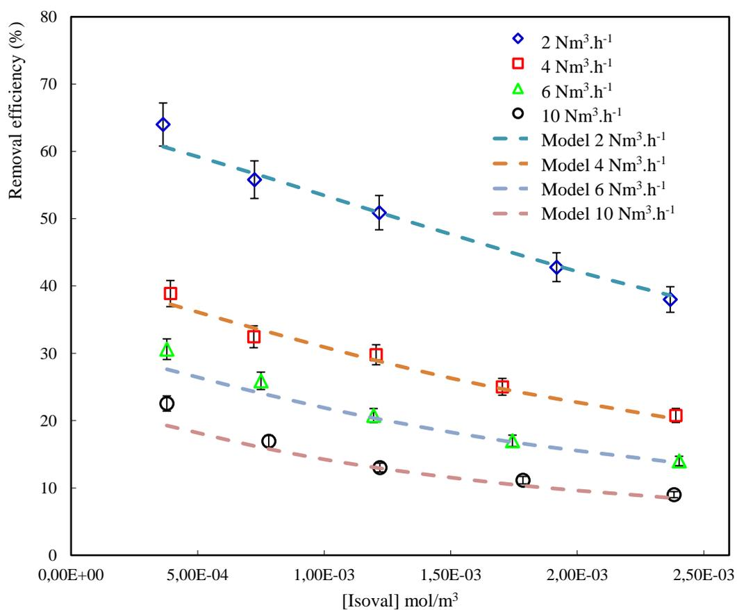
Fig. 7: Variation of removal efficiency of isovaleraldehyde with the inlet concentration at different flowrates in cylindrical reactor ( $T = 20^{\circ}\text{C}$ ,  $\text{RH} = 50\%$ ,  $I = 24\text{W}\cdot\text{m}^{-2}$ )
