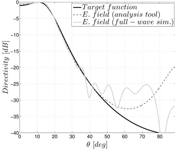
Fig. 2. Flat-topped radiation pattern in E-plane ( $\phi = 90^\circ$ ). The black curve represents the analytical function to be approximated. The normalized far-field radiation pattern of the optimized structure evaluated using the in-house analysis tool and full-wave simulations are shown in dashed gray line and solid gray curve, respectively.
