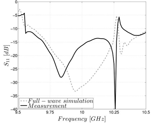
Fig. 5. Simulated and measured reflection coefficient.
