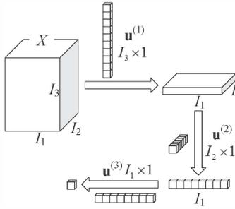
**Fig. 1.** The process of elementary multilinear projection (EMP).
