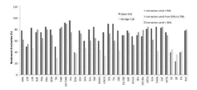
Figure 1: Extraction yields calculated for the two cartridges (Oasis HLB and Xbridge C18) tested for all molecules in neutral pH
