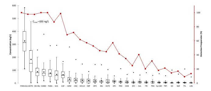
Figure 7: overall mean concentrations (\*), median value, first and third quartiles and extrema of 27 molecules detected on average above LOQ in surface waters and detection frequencies (%, broken line).
