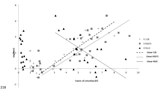
Figure 3: Polarity (log Kow) as function of the capacity factor for all molecules and for 3 chromatographic columns
