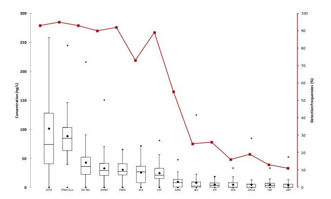
Figure 8: overall mean concentrations(♦), median value, first and third quartiles and extrema for 14 molecules detected in tap waters and detection frequencies (%, broken line).
