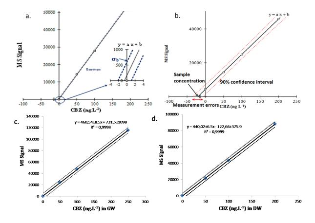
Figure 5: a. equation of LOQ determanation. b. Exemple of standard addition for CBZ with 90% confidence interval. c. and d. Exemple of standard addition in GW and DW for CBZ
