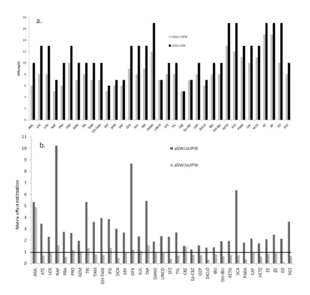
Figure 6: a. LOQ in UPW and GW for all molecules b. Matrix effects of all analytes
