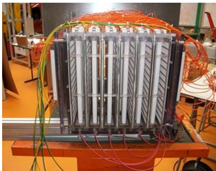
Photograph of prototype combining plasma and photocatalysis in situ
