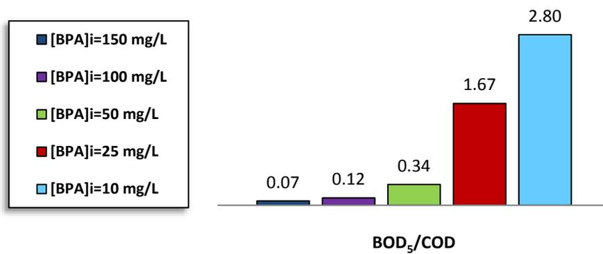
Fig. 11: Variation of BOD<sub>5</sub>/COD ratio according to the initial concentration of BPA after 90 min of treatment by electro-Fenton process. Experimental conditions: I= 0.8 A, [FeSO<sub>4</sub>] = 0.5 mM, [Na<sub>2</sub>SO<sub>4</sub>] =0.05 M, pH = 2.9 ± 0.1, Flow rate = 6 L.min<sup>-1</sup>
