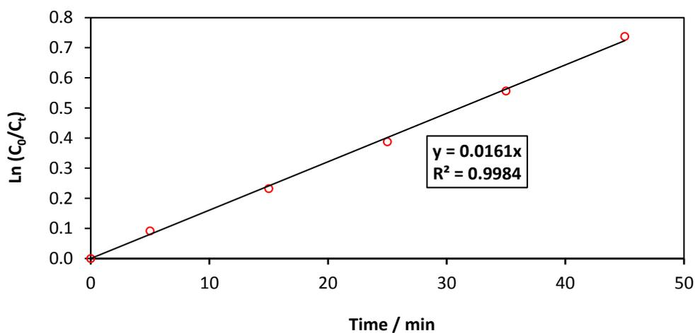
Fig. 8: Variation of  $\ln(C_0/C_t)$  functions to time during treatment of BPA by electro-Fenton process. Experimental conditions:  $I = 0.8$  A,  $[\text{BPA}] = 150 \text{ mg}\cdot\text{L}^{-1}$ ,  $[\text{FeSO}_4] = 0.5$  mM,  $[\text{Na}_2\text{SO}_4] = 0.05$  M,  $\text{pH} = 2.9 \pm 0.1$ , Flow rate =  $6 \text{ L}\cdot\text{min}^{-1}$
