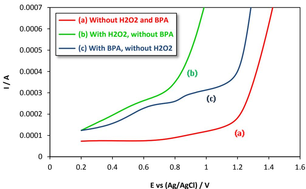
Fig. 5: Cyclic voltammograms of H<sub>2</sub>O<sub>2</sub> and BPA at DSA microelectrode material. Experimental conditions: [Na<sub>2</sub>SO<sub>4</sub>] = 0.05 M, pH = 2.9 ± 0.1, v = 0.05 V/s
