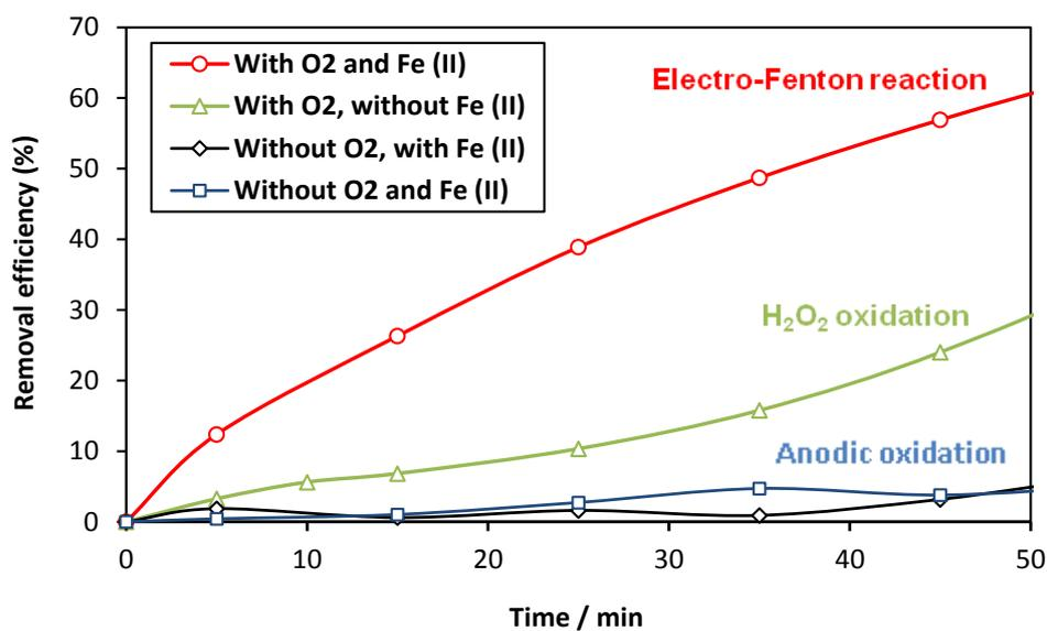
Fig. 6: Evolution of the removal efficiency of BPA by electrolysis in presence/absence of O<sub>2</sub> and Fe<sup>II</sup>. Experimental conditions: I = 0.8 A, [BPA] = 150 mg.L<sup>-1</sup>, [FeSO<sub>4</sub>] = 0.5 mM, [Na<sub>2</sub>SO<sub>4</sub>] = 0.05 M, pH = 2.9 ± 0.1, Flow rate = 6 L.min<sup>-1</sup>
