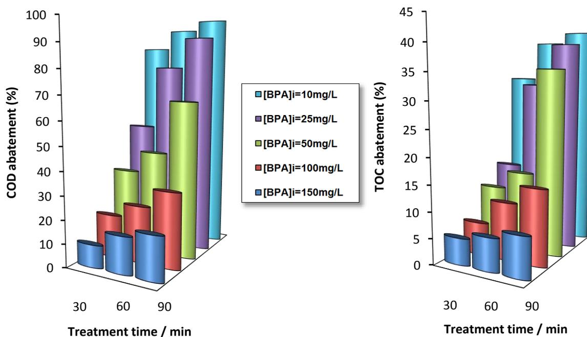
**Fig. 10: COD and TOC abatement during treatment of BPA by electro-Fenton process at different time. Experimental conditions:  $I = 0.8$  A,  $[FeSO_4] = 0.5$  mM,  $[Na_2SO_4] = 0.05$  M,  $pH = 2.9 \pm 0.1$ , Flow rate =  $6$  L.min $^{-1}$**
