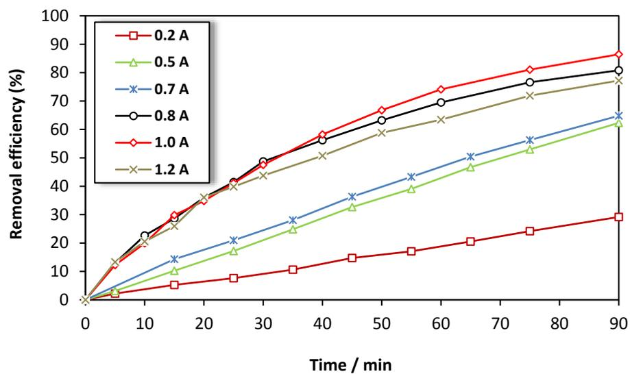
**Fig. 2:** Effect of the applied current intensity on the removal efficiency of BPA for treatments by electro-Fenton process. Experimental conditions: [BPA] = 150 mg.L<sup>-1</sup>, [FeSO<sub>4</sub>] = 0.5 mM, [Na<sub>2</sub>SO<sub>4</sub>] = 0.05 M, pH = 2.9 ± 0.1, Flow rate = 6 L.min<sup>-1</sup>
