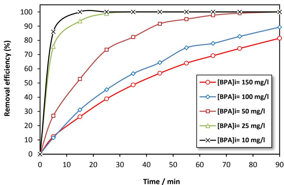
Fig. 7: Effect of the initial concentration of BPA on the degradation kinetics by electro-Fenton process. Experimental conditions:  $I = 0.8$  A,  $[\text{FeSO}_4] = 0.5$  mM,  $[\text{Na}_2\text{SO}_4] = 0.05$  M,  $\text{pH} = 2.9 \pm 0.1$ , Flow rate =  $6 \text{ L}\cdot\text{min}^{-1}$
