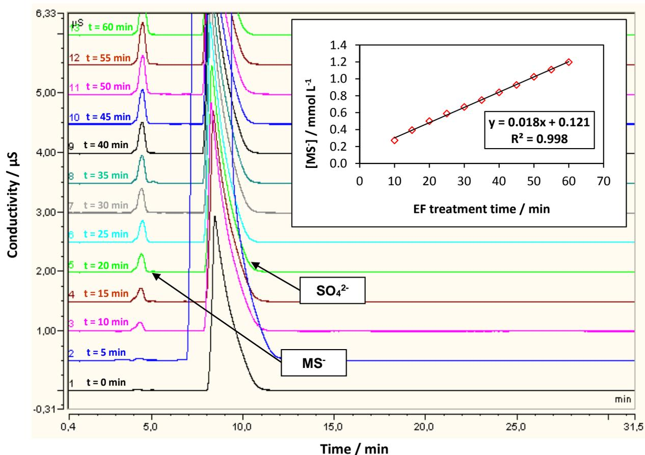
Fig. 4: Monitoring of methanesulfonate production by ion chromatography during electro-Fenton process with DMSO as molecular probe of  $\cdot$ OH production. Experimental conditions: I = 0.8 A, [FeSO<sub>4</sub>] = 0.5 mM, [Na<sub>2</sub>SO<sub>4</sub>] = 1mM, pH = 2.9 ± 0.1, Flow rate = 6 L.min<sup>-1</sup>
