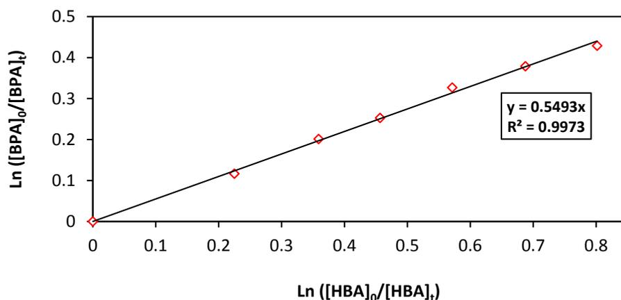
**Fig. 9: Competitive method for kinetic analysis of BPA oxidation by the hydroxyl radicals' electro-generated by electro-Fenton process. Experimental conditions:  $I = 0.8$  A,  $[BPA] = [HBA] = 0.65$  mM,  $[FeSO_4] = 0.5$  mM,  $[Na_2SO_4] = 0.05$  M,  $pH = 2.9 \pm 0.1$ , Flow rate =  $6$  L.min $^{-1}$ , Time = 30 min**
