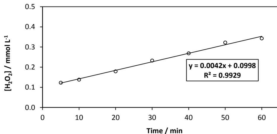
Fig. 3: Production of H<sub>2</sub>O<sub>2</sub> during electro-Fenton process in absence of Fe<sup>II</sup>. Experimental conditions: I = 0.8 A, [Na<sub>2</sub>SO<sub>4</sub>] = 0.05 M, pH = 2.9 ± 0.1, Flow rate = 6 L.min<sup>-1</sup>
