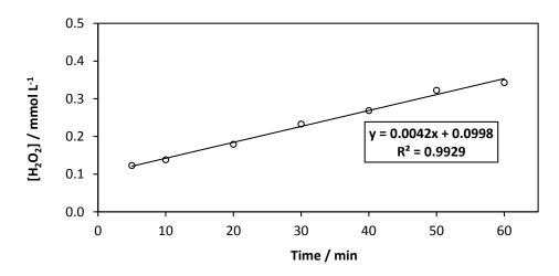
Fig. 3: Production of  $H_2O_2$  during electro-Fenton process in absence of  $Fe^{II}$ . Experimental conditions: I= 0.8 A, [Na<sub>2</sub>SO<sub>4</sub>] =0.05 M, pH = 2.9 ± 0.1, Flow rate = 6 L.min<sup>-1</sup>
