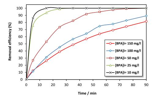
Fig. 7: Effect of the initial concentration of BPA on the degradation kinetics by electro-Fenton process. Experimental conditions: I= 0.8 A, [FeSO<sub>4</sub>] = 0.5 mM, [Na<sub>2</sub>SO<sub>4</sub>] =0.05 M, pH =  $2.9 \pm 0.1$ , Flow rate = 6 L.min<sup>-1</sup>
