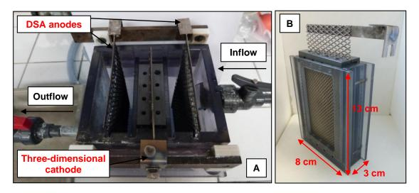
Fig. 1: Pictures of the open one-compartment electrochemical reactor for the application of electro-Fenton process (A) and the associated fixed bed three-dimensional cathode (B)
