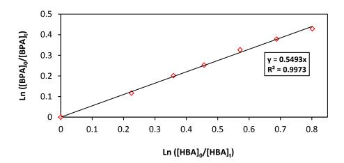
Fig. 9: Competitive method for kinetic analysis of BPA oxidation by the hydroxyl radicals' electro-generated by electro-Fenton process. Experimental conditions: I= 0.8 A, [BPA] = [HBA] = 0.65 mM,  $[FeSO_4] = 0.5 \text{ mM}$ ,  $[Na_2SO_4] = 0.05 \text{ M}$ ,  $pH = 2.9 \pm 0.1$ , Flow rate = 6 L.min<sup>-1</sup>, Time = 30 min
