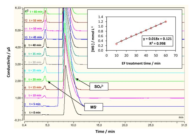
Fig. 4: Monitoring of methanesulfonate production by ion chromatography during electro-Fenton process with DMSO as molecular probe of 'OH production. Experimental conditions: I= 0.8 A, [FeSO<sub>4</sub>] = 0.5 mM, [Na<sub>2</sub>SO<sub>4</sub>] =1mM, pH =  $2.9 \pm 0.1$ , Flow rate = 6 L.min<sup>-1</sup>
