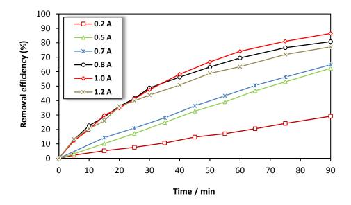
Fig. 2: Effect of the applied current intensity on the removal efficiency of BPA for treatments by electro-Fenton process. Experimental conditions:  $[BPA] = 150 \text{ mg.L}^{-1}$ ,  $[FeSO_4] = 0.5 \text{ mM}$ ,  $[Na_2SO_4] = 0.05 \text{ M}$ ,  $pH = 2.9 \pm 0.1$ , Flow rate = 6 L.min<sup>-1</sup>
