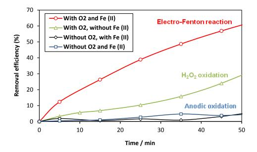
Fig. 6: Evolution of the removal efficiency of BPA by electrolysis in presence/absence of  $O_2$  and Fe<sup>II</sup>. Experimental conditions: I= 0.8 A, [BPA] = 150 mg.L<sup>-1</sup>, [FeSO<sub>4</sub>] = 0.5 mM, [Na<sub>2</sub>SO<sub>4</sub>] =0.05 M, pH =  $2.9 \pm 0.1$ , Flow rate = 6 L.min<sup>-1</sup>
