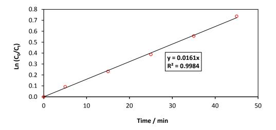
Fig. 8: Variation of Ln (C<sub>0</sub>/C<sub>t</sub>) functions to time during treatment of BPA by electro-Fenton process. Experimental conditions: I= 0.8 A,[BPA] = 150 mg.L<sup>-1</sup>, [FeSO<sub>4</sub>] = 0.5 mM, [Na<sub>2</sub>SO<sub>4</sub>] = 0.05 M, pH =  $2.9 \pm 0.1$ , Flow rate = 6 L.min<sup>-1</sup>
