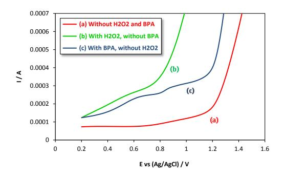
Fig. 5: Cyclic voltammograms of H<sub>2</sub>O<sub>2</sub> and BPA at DSA microelectrode material. Experimental conditions: [Na<sub>2</sub>SO<sub>4</sub>] =0.05 M, pH =  $2.9 \pm 0.1$ , v= 0.05 V/s
