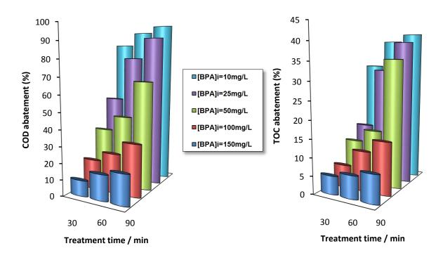
Fig. 10: COD and TOC abatement during treatment of BPA by electro-Fenton process at different time. Experimental conditions: I= 0.8 A, [FeSO<sub>4</sub>] = 0.5 mM, [Na<sub>2</sub>SO<sub>4</sub>] =0.05 M, pH = 2.9  $\pm$  0.1, Flow rate = 6 L.min<sup>-1</sup>
