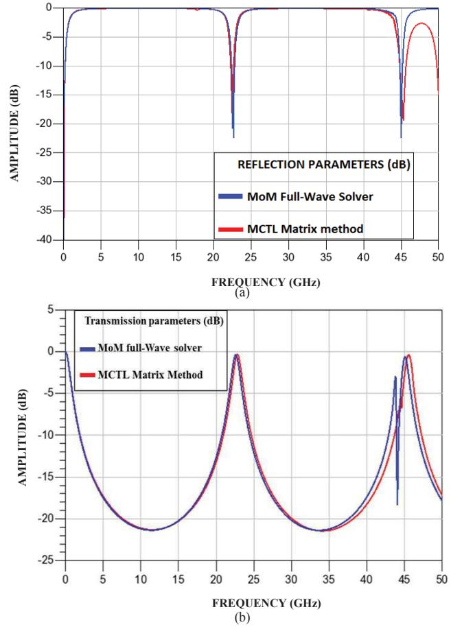
**Fig.13: Simulated and modeled S-parameters for three-layered Power/Ground planes (a) Reflection parameters; (b) Transmission parameters. The results are very close but the computation time is much lower.**
