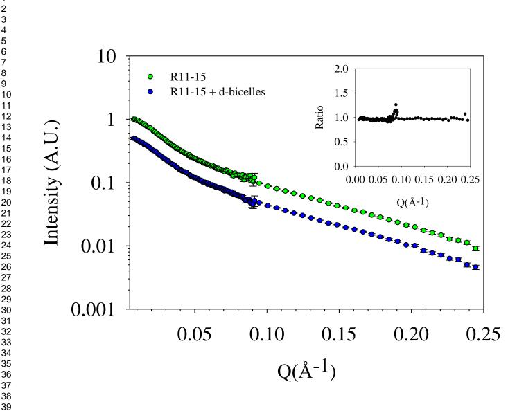
Figure 5: Normalized SANS intensities measured for DYS R11-15 at 93 µM (5.6 g/L) alone (green) or in the presence of the d-bicelles (blue) in 100% D<sub>2</sub>O d-TNE at 18°C. Insert: the ratio of the two scattering curves. The blue curve is shifted for clarity since the two curves superimpose, as shown by the ratio of the raw data in the insert.
