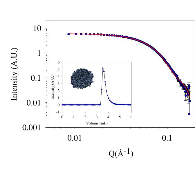
Figure 6: HPSEC-SANS intensities measured for h-bicelles fitted (red line) with the expected "core-shell cylinder" model as for the same sample in the Hellma cell environment. Insert: the associated scattergram (SANS detector) as a function of elution volume, showing one unique peak corresponding to h-bicelles.
