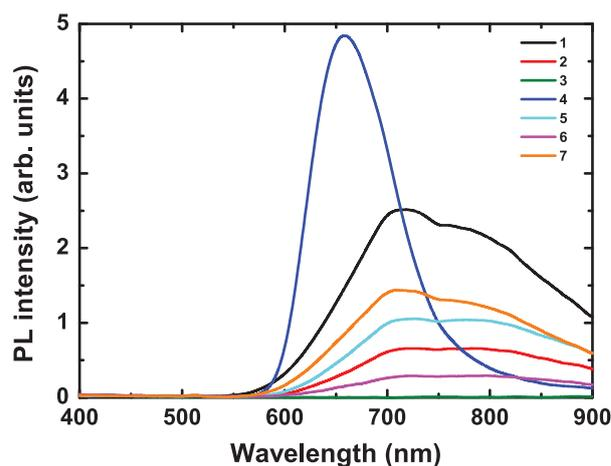
Figure 2. PL spectra of 1–7 compound series ( $\lambda_{\text{exc}} = 325$  nm).
