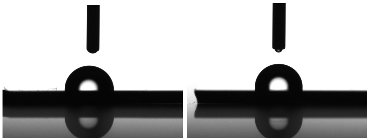
Figure S2. Profile of a \text{H}_2\text{O} droplet in contact with a SAM of complex 6o (left) and 8o (right) on gold
