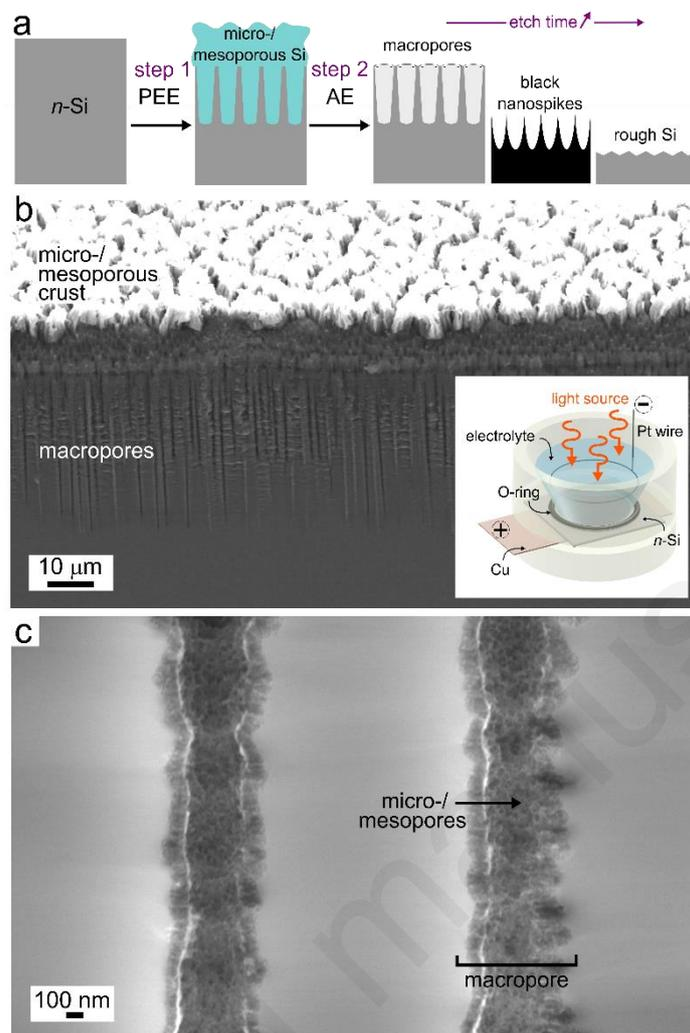
**Figure 1.** a) Two-step structuration procedure involving a first photoelectrochemical etching (PEE) followed by an alkaline etching (AE). b) Low magnification tilted view (45°) showing the macropores covered by a micro-/mesoporous transitional layer (Si layer obtained after a PEE of 4 min at  $0.13 \text{ A cm}^{-2}$ ). Inset: Scheme of the photoelectrochemical setup used for PEE. c) High magnification cross-section showing the inner walls of two macropores.
