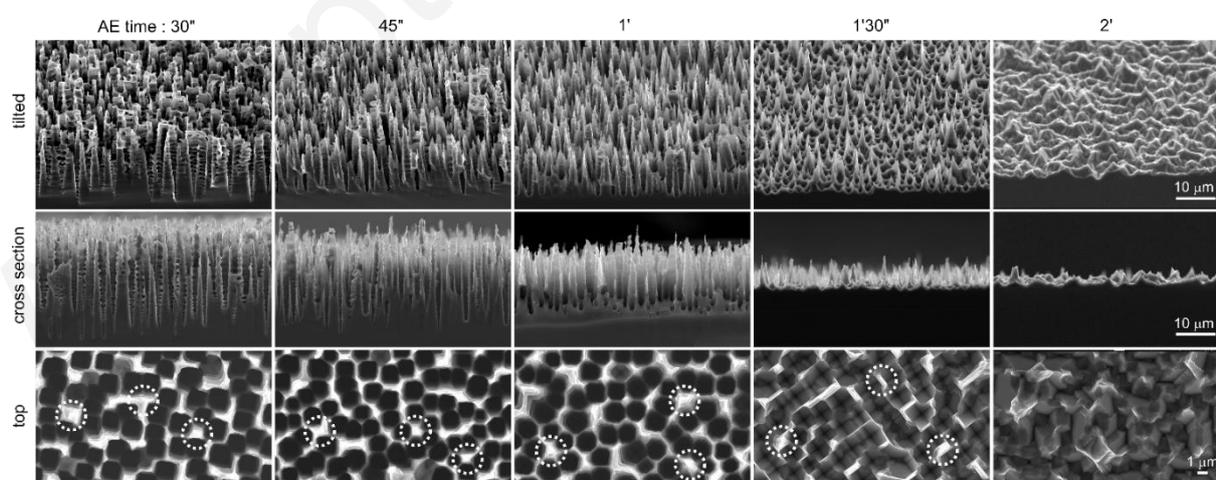
**Figure 2.** SEM images showing the Si porous layer obtained after different times of AE (note that in all cases, the surface was patterned with an identical PEE step of 4 min at  $0.13 \text{ A cm}^{-2}$ ). The time of AE is indicated on the top of each column. Top, middle and bottom rows show tilted ( $45^\circ$ ), cross-section and
