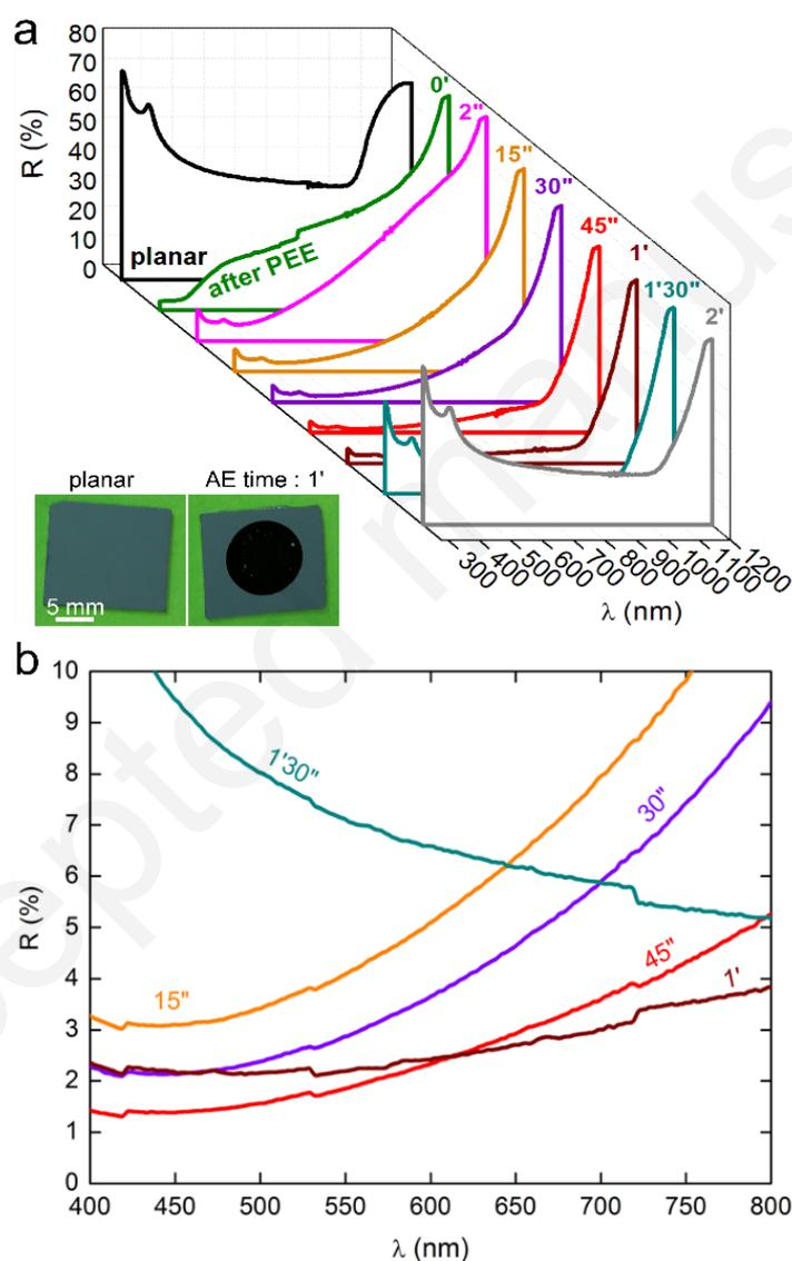
**Figure 3.** a) Series of UV-vis-NIR total reflectance spectra showing the evolution of the reflectance as a function of the AE time. Inset: Photograph of a planar Si surface (left) and a Si NSpike surface (right). b) Reflectance in the visible range for the most absorbing samples.
