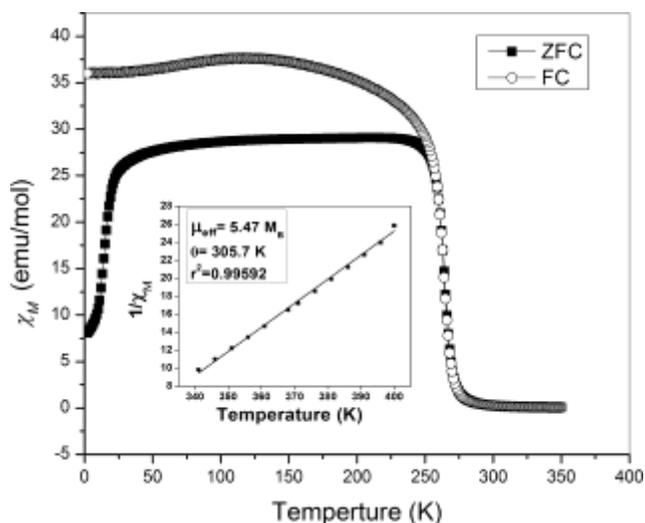
**Figure 6:** ZFC/FC magnetization cycles measured at  $H_{app} = 500$  Oe for a powder sample of  $CuCr_{1.3}Sn_{0.7}Se_4$ . The insert shows the  $1/\chi$ -versus-temperature behavior fitted by a Curie-Weiss law.
