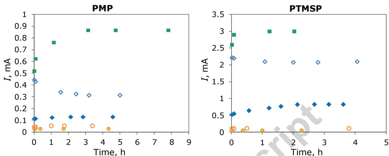
Fig 3. The change of the AC through system over the time (with PMP and PTMSP membrane) with different liquids at 1000 Hz ( $C_{\text{NaCl}}=0.5$  g/L); ■ – ethanol; ◇ – 60% ethanol (W-E); ◆ – 60% ethanol (E-W); ● – water (initial); ○ – water (after ethanol).
