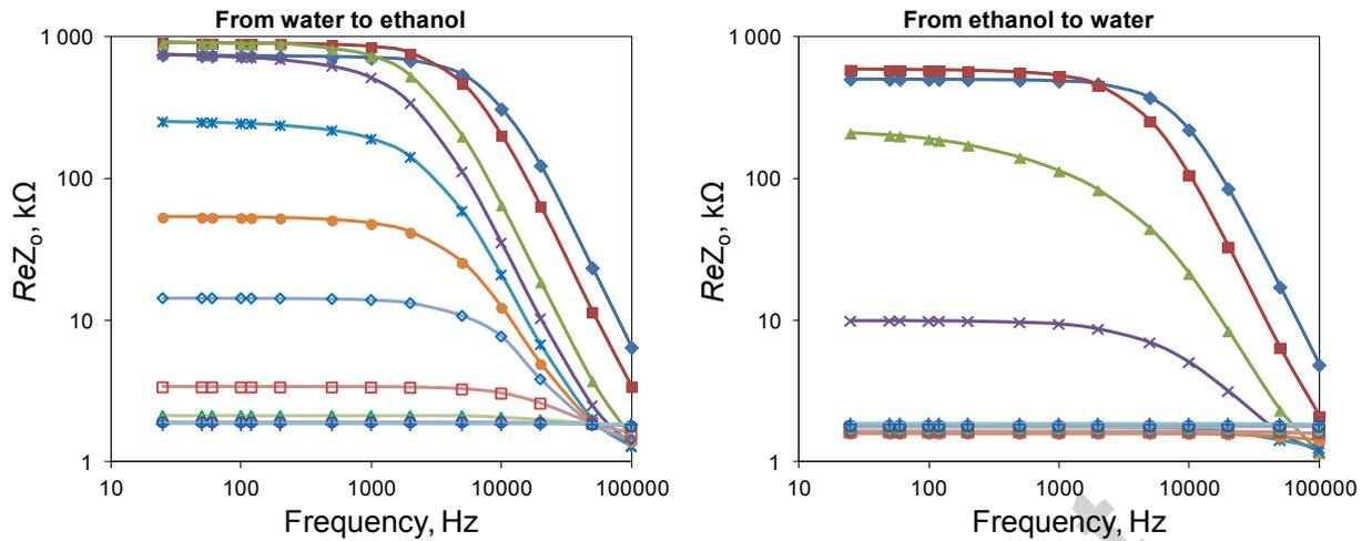
Fig A-4. Experimentally measured real part of impedance of system consists of PTMSP membrane and water-ethanol solutions  $ReZ_0$ . ◆ – water, ■ – 10% ethanol; ▲ – 20% ethanol; × – 30% ethanol; \* – 40% ethanol; ● – 50% ethanol; ◇ – 60% ethanol; □ – 70% ethanol; Δ – 80% ethanol; ○ – 90% ethanol; + – 96% ethanol.
