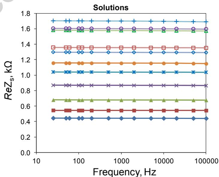
Fig A-1. Experimentally measured real part of impedance of water-ethanol solutions  $ReZ_s$ .
