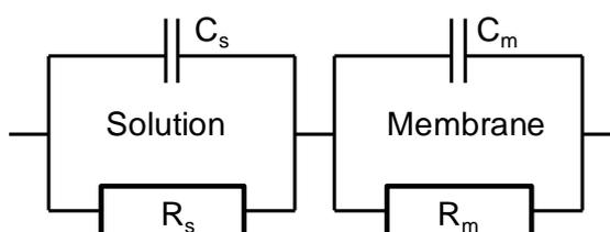
Fig 2. Equivalent circuit of experimental setup.
