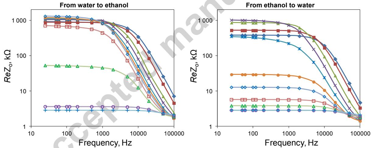
Fig A-7. Experimentally measured real part of impedance of system consists of PMP membrane and water-ethanol solutions  $ReZ_o$ .  $\blacklozenge$  – water,  $\blacksquare$  – 10% ethanol;  $\blacktriangle$  – 20% ethanol;  $\times$  – 30% ethanol;  $*$  – 40% ethanol;  $\bullet$  – 50% ethanol;  $\blacklozenge$  – 60% ethanol;  $\square$  – 70% ethanol;  $\blacktriangle$  – 80% ethanol;  $\circ$  – 90% ethanol;  $+$  – 96% ethanol.
