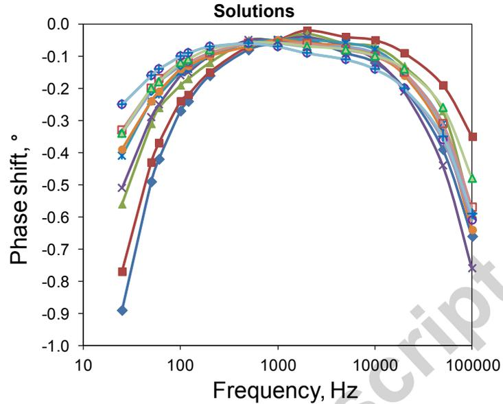
Fig A-2. Experimentally measured phase shift in water-ethanol solutions  $\varphi_s$ .
