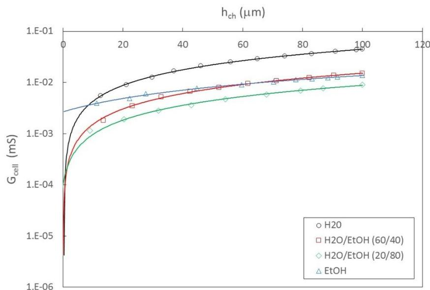
Fig 7. Variation of the cell conductance ( $G_{\text{cell}}$ ) as a function of the gap between membrane samples ( $h_{\text{ch}}$ ) in the lateral-measurement configuration with the PMP membrane.
