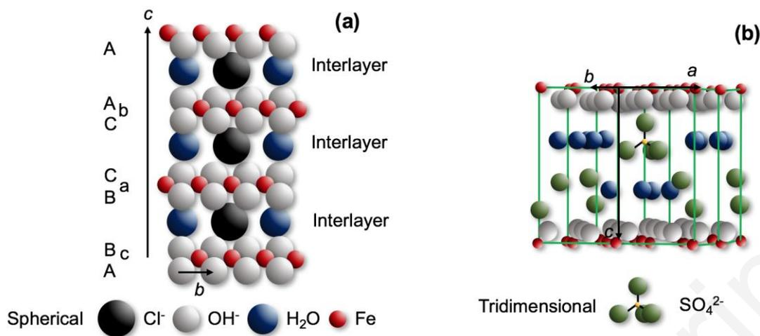
**Figure 2:** General view of the crystal structure of green rusts: (a) GR-I (Cl<sup>-</sup>) (b) GR-II (SO<sub>4</sub><sup>2-</sup>). Image (a) is adapted with permission from Ref. 26. Copyright 1998 Elsevier. Image (b) is adapted with permission from Ref. 24. Copyright 2003 Elsevier Masson SAS.
