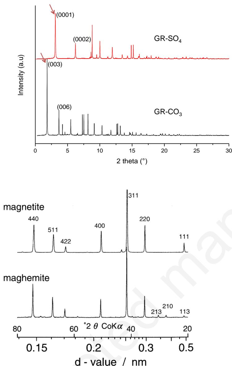
**Figure 12.** X-ray diffractograms of green rusts namely GR(SO<sub>4</sub><sup>2-</sup>) and GR(CO<sub>3</sub><sup>2-</sup>), magnetite, and maghemite. Diffractograms of GR(SO<sub>4</sub><sup>2-</sup>) and GR(CO<sub>3</sub><sup>2-</sup>) are reproduced with permission from Ref. 19. Copyright 2010 Elsevier. Diffractograms of magnetite and maghemite are reproduced with permission from Ref. 2. Copyright 2003 Wiley-VCH Verlag GmbH & Co. KGaA.
