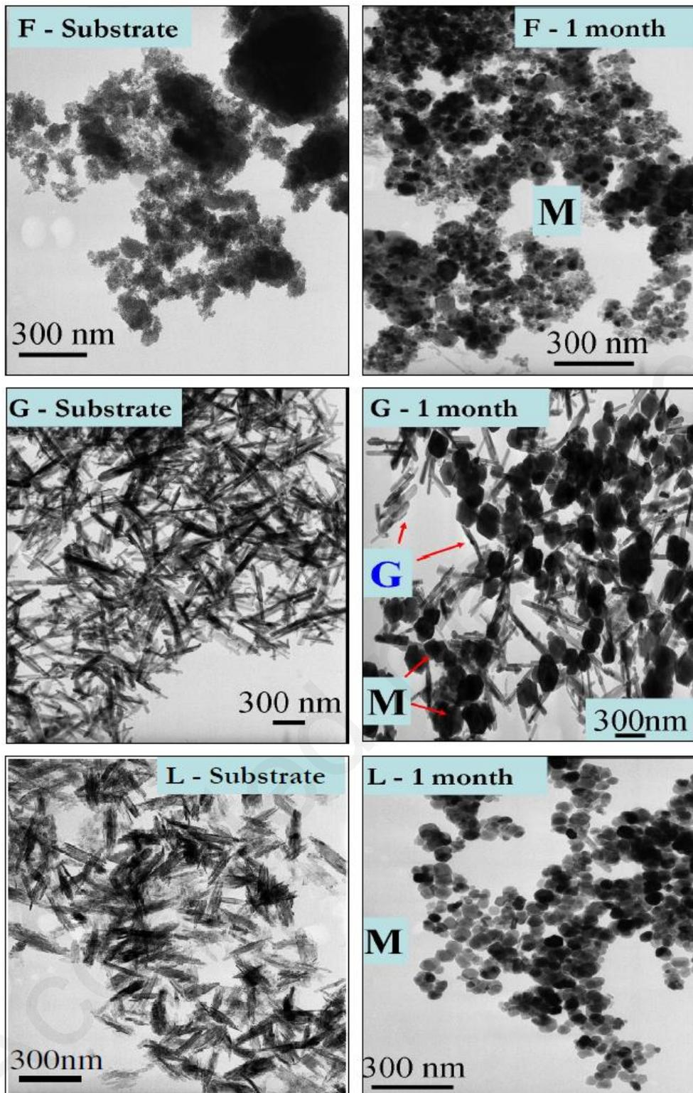
**Figure 8:** Bright field transmission electron microscopy images showing initial ferric (oxyhydr)oxides (ferrihydrite-F, lepidocrocite-L and goethite-G) and their transformations products after their reaction with suitable amounts of Fe(II) and OH<sup>-</sup> to form stoichiometric magnetite (M). Transformation product of G indicates the presence of M and untransformed G. Reproduced with permission from Ref. 37. Copyright 2012 Elsevier.
