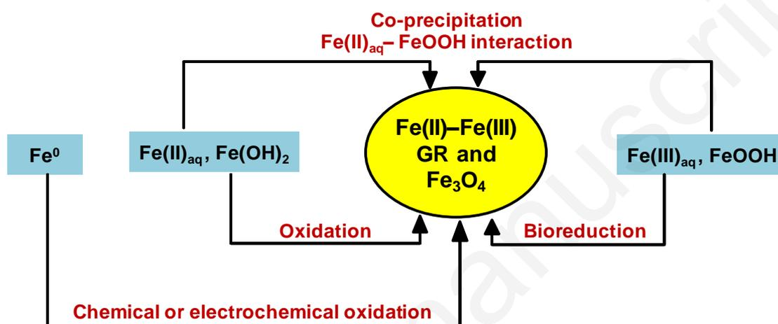
**Figure 5:** Overview of different pathways for the formation of magnetite (Fe<sub>3</sub>O<sub>4</sub>) and green rust (GR).
