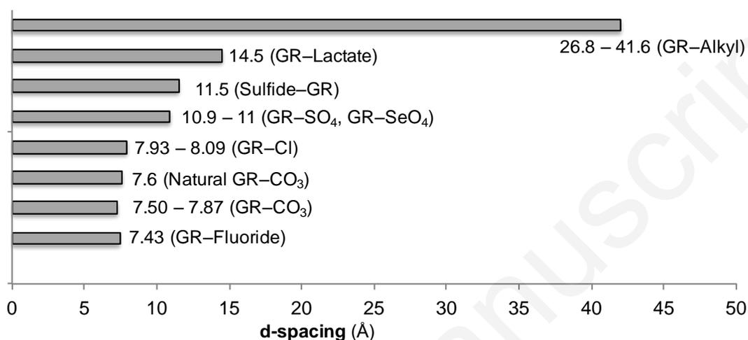
**Figure 13:** Variation of  $d$ -spacings in XRD parameters of different GRs depending upon their type and nature of intercalated molecules. This figure is based on the data compiled in previous studies<sup>22,26,88,331,332</sup> and references cited therein.
