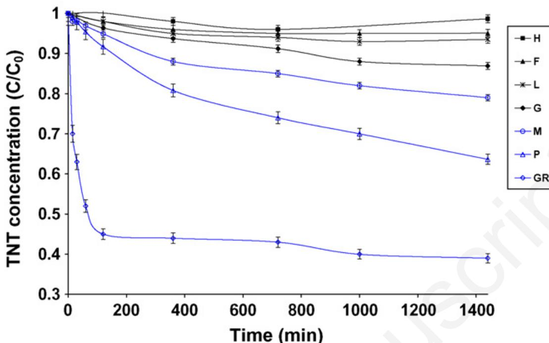
**Figure 22:** Fenton-like oxidation of TNT (0.11 mM) in the presence of six different iron minerals (2 g L<sup>-1</sup>) at pH 7: (■) hematite, (▲) ferrihydrite, (\*) lepidocrocite, (◆) goethite, (○) magnetite, (△) pyrite, (◇) green rust. H<sub>2</sub>O<sub>2</sub> (3%, w/v). Reproduced with permission from Ref. 504. Copyright 2008 Elsevier.
