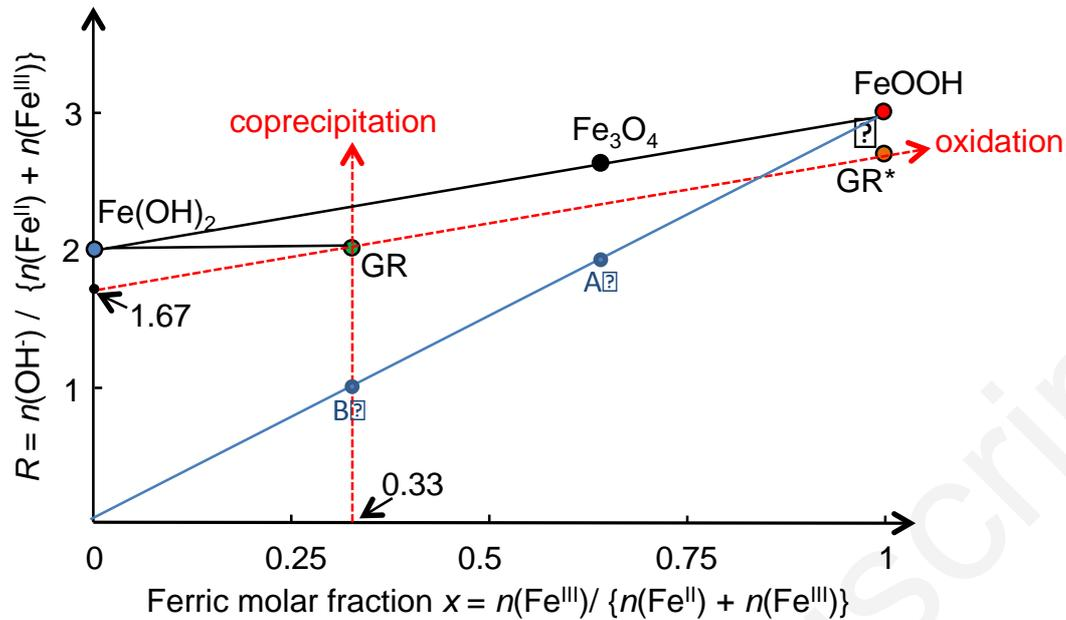
**Figure 6:** The mass-balance diagram representing the synthesis of magnetite ( $\text{Fe}_3\text{O}_4$ ) and green rust *via* co-precipitation and oxidation. GR correspond to green rust and GR\* to the fully oxidized form of GR, *i.e.* Mössbauerite. Point A correspond to the mixture [2/3 FeOOH, 1/3 Fe(II)] and point B is mixture [1/3 FeOOH, 2/3 Fe(II)]. Adapted with permission from Ref. 31. Copyright 2006 Elsevier Masson SAS.
