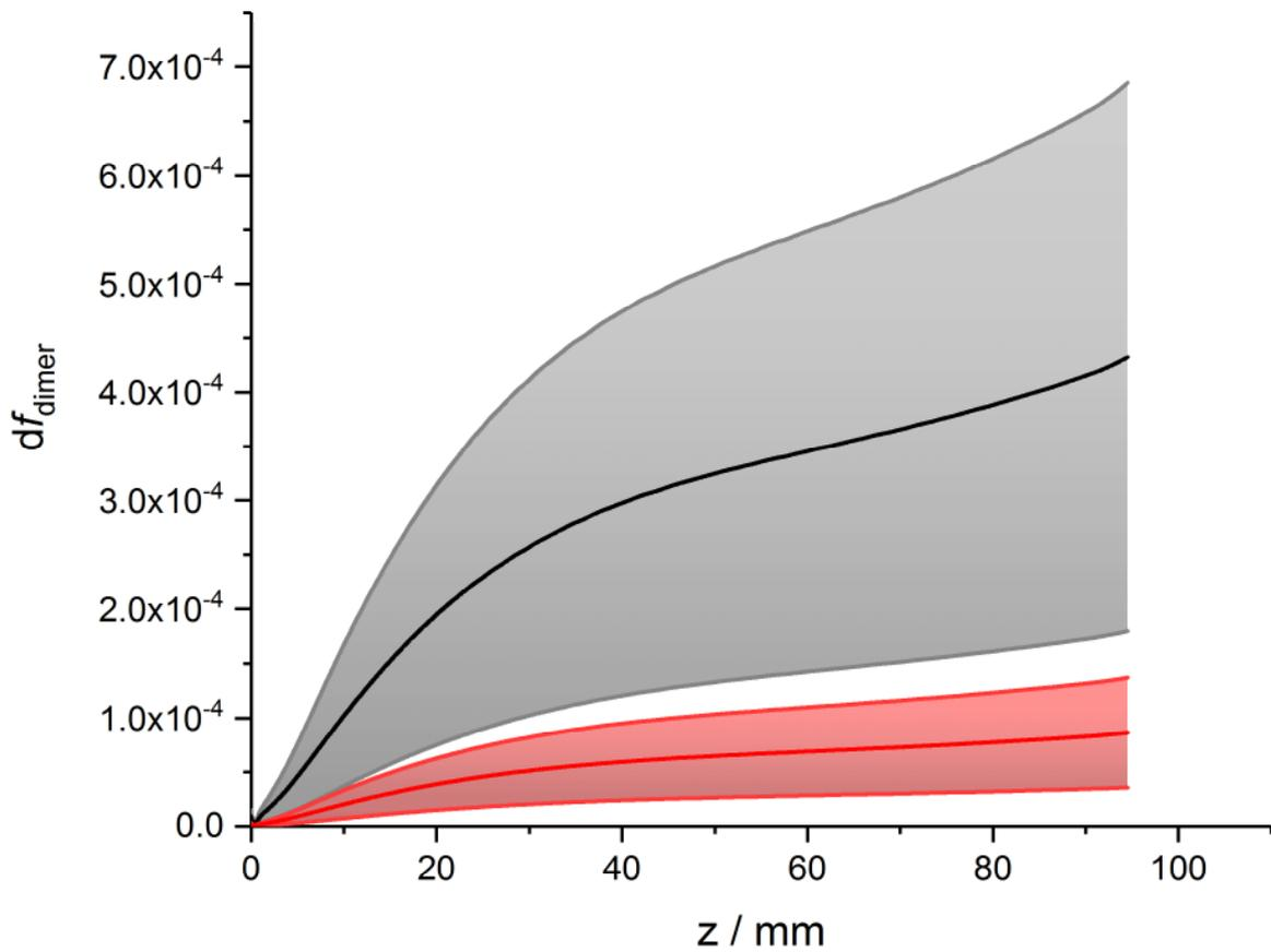
**Figure 1.** Calculated  $df_{\text{dimer}}$  as a function of the distance along the 52 K Laval nozzle axis ( $z$ ) from throat to nozzle exit. The black line assumes 0.5% of the gas flow consists of methanol (the maximum used with this nozzle) whilst the red line assumes 0.1% of the total gas flow consists of methanol. Error bars are assigned through varying the binding energy of the dimer as described in Section 2 of the manuscript.
