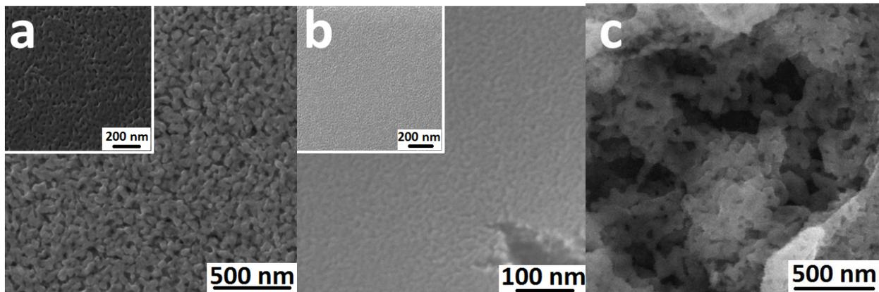
**Figure 1.** Surface morphology of (a) pristine  $\text{BiVO}_4$  and (inset) top-coated  $\text{BiVO}_4$  over  $\text{TiO}_2$  composite, (b) pure  $\text{TiO}_2$  and (inset) top-coated  $\text{TiO}_2$  over  $\text{BiVO}_4$  composite and (c)  $\text{Nb-BiVO}_4$ .
