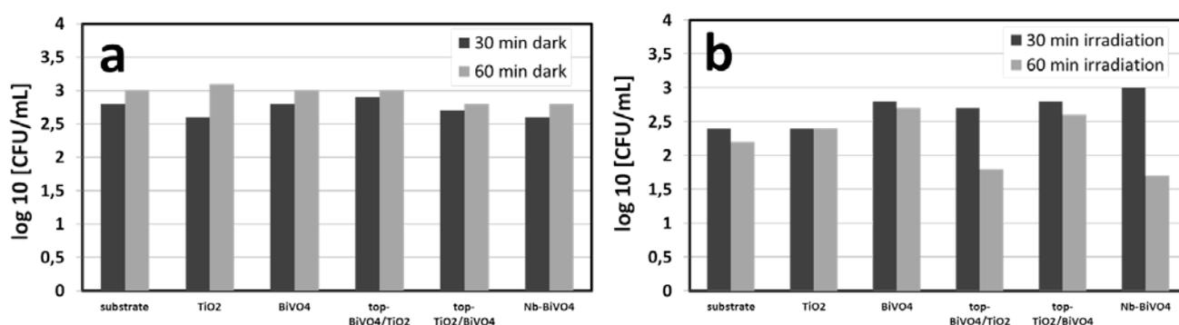
**Figure 3.** Survival of MRSA strain on the different BiVO<sub>4</sub>-based materials (a) in the dark, (b) after 30 and 60min solar-like irradiation.
