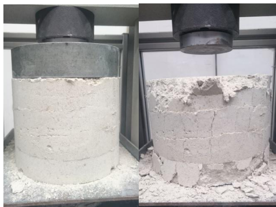
295 Fig. 9: Observation of the dynamically compacted samples with 4 woven fabric sheets before 296 and after the compressive strength test.
