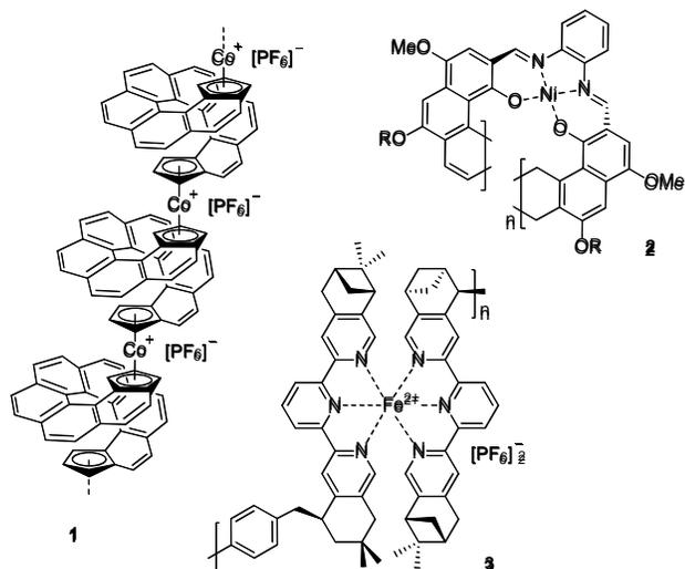
**Figure 1.** Metal-containing chiral oligomers and coordination polymers 1-3.
