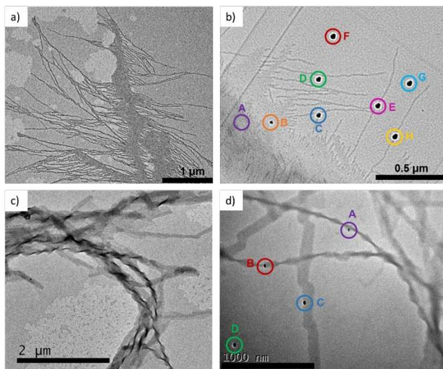
**Figure 7.** TEM images obtained after drop-casting an aliquot of solutions of  $[PCE][C_{16-L-Ala}]_n$  complex in a) ethanol (ca. 12 mg mL<sup>-1</sup>) and b) spot EDX analyses of film and fibrous material (drop cast from 12 mg mL<sup>-1</sup> ethanolic solution), or c) by drop-casting suspensions of  $[PCE][C_{16-L-Ala}]_n$  assemblies in water, and d) spot EDX analyses of helices. For detailed EDX analysis of spots see Supporting Information (Figs. S9 and S28).
