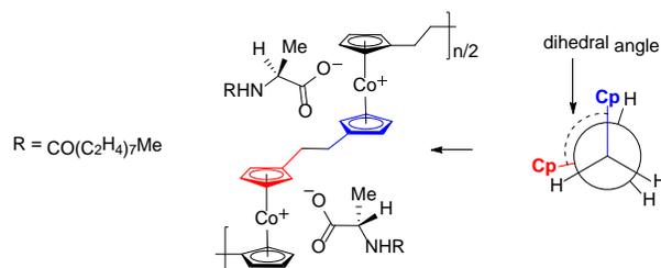
**Figure 6.** Structure of [PCE][C<sub>16</sub>-L-Ala]<sub>n</sub> with example Newman projection along the CH<sub>2</sub>-CH<sub>2</sub> axis to demonstrate chirality of the polymer backbone.
