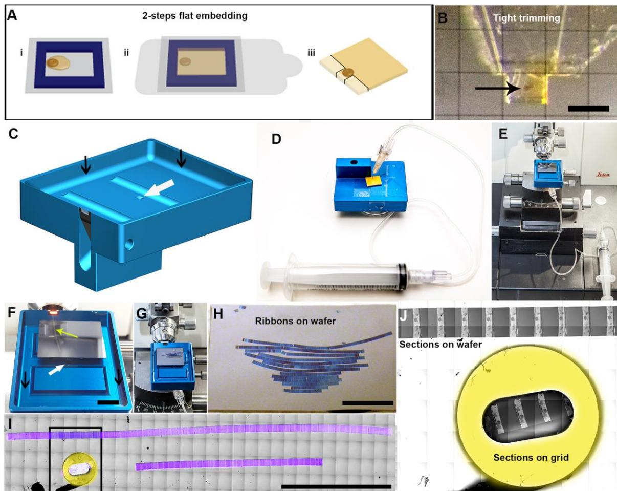
**Figure 1, AT: Generation of arrays of aligned ribbons of consecutive sections**
