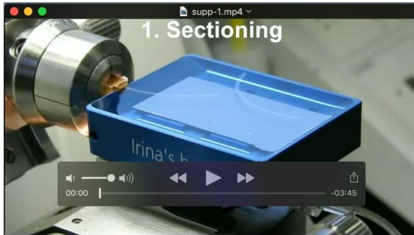
**Movie 1.** Sectioning and on-wafer transfer of the arrays using the modified diamond knife with the modified basin. There are several key steps in this procedure:
