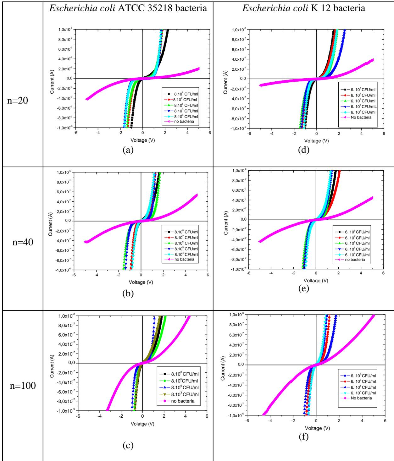
Figure 5: I-V curves of the SiNWs based resistors with  $n = 20, 40, 100$  teeth and  $5 \mu\text{m}$  interspacing, after *Escherichia coli* ATCC 35218 immobilization (a), (b), (c), and *Escherichia coli* K12 bacteria immobilization (d), (e), (f). Curves for devices submitted to a mixture of distilled water and culture solution without bacteria are given as reference.
