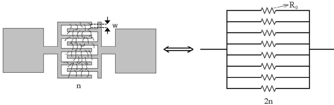
Figure 2: Equivalent circuit diagram of SiNWs based resistors
