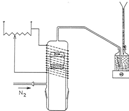
**Figure 1.** Device used for nitrogen determination.
