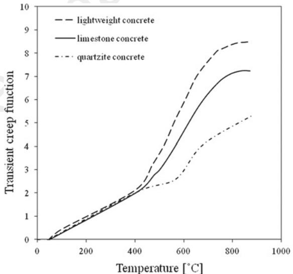
exceeding this level, it increases more rapidly for the concrete with siliceous type of aggregates (Seine gravel).
