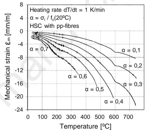
from the thermal strains under load. It can be observed, that thermal strains of those two concretes are close due to the type of aggregates used for both concretes. From 20 °C to about 400 °C, the thermal strain curves are almost linear. Above 400 °C strains increase more rapidly due to crack development.
