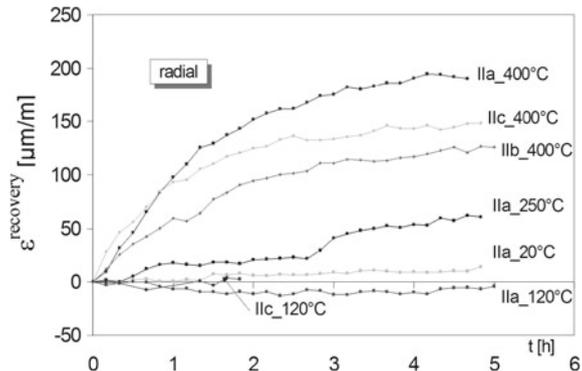
**Fig. 5.35** Creep recovery strain of sealed basalt concrete samples at 20 °C (Schneider 1982)
