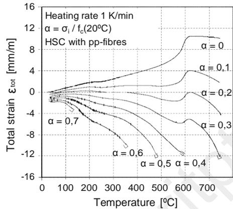
**Fig. 5.43** Transient thermal strain under load of high strength concrete with PP fibres (Huismann 2010)
