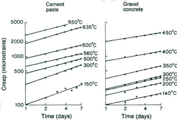
**Fig. 5.32** Drying creep of high performance cement paste and gravel concrete (Khoury et al. 1986)
