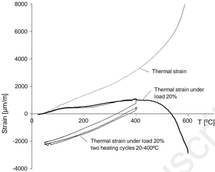
**Fig. 5.52** Thermal strain under load curves of HPC sample after two cycles of heating at 400 °C (Hager 2004)
