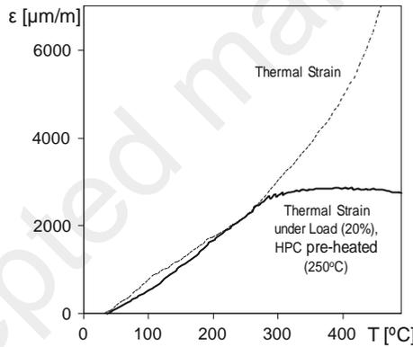
**Fig. 5.53** Thermal strain and thermal strain under load of HPC in a sample pre-heated up to 250 °C, transient thermal strain is re-activated when  $T > 250$  °C (Hager 2004)
