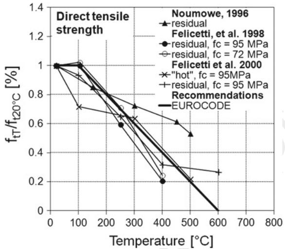
of the tensile strength with temperature in the range 20–400 °C. Such behaviour has been explained by the drying processes that increase the strength of concrete. From the results presenting direct hot and residual results (Felicetti and Gambarova 1998), it can also be concluded that values obtained for hot specimens are lower than those obtained after cooling them down (Felicetti et al. 2000).
