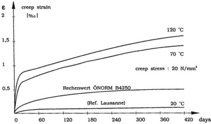
**Fig. 5.24** Basic creep of high performance basalt concrete; samples tested in autoclave (concrete tested at age of 90 days) (Schneider 1982)
