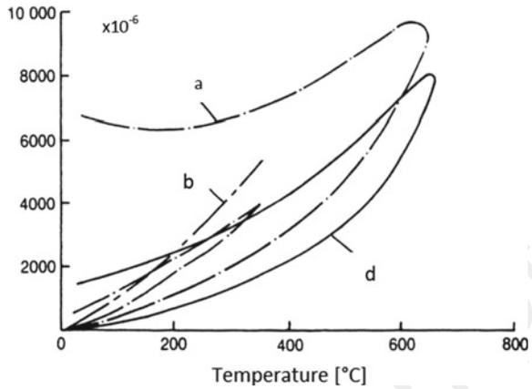
**Fig. 5.37** Thermal strain of aggregates; a and g—sandstone, b and f—calcareous, c—granite, d—anorthosite, e—basalt and h—pumice (Bažant and Kaplan 1996)
