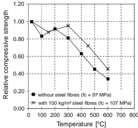
**Fig. 5.10** Compressive strength of HPC with and without steel fibres according to Huismann et al. (2007)
