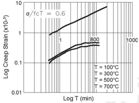
**Fig. 5.27** Effect of stress ratio on drying creep of HPC (84 MPa) with PP fibres at 700 °C. Load levels of 0.2, 0.4, and 0.6 (Wu et al. 2010)
