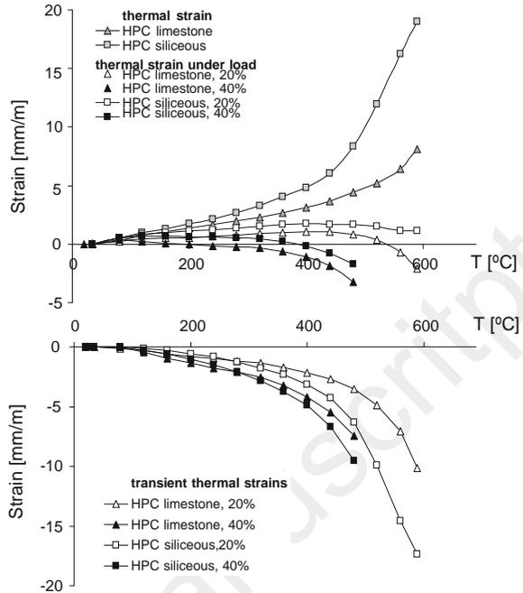
**Fig. 5.46** Transient thermal strains (transient creep—Schneider’s nomenclature) of concretes with different type of aggregates (Schneider 1988)
