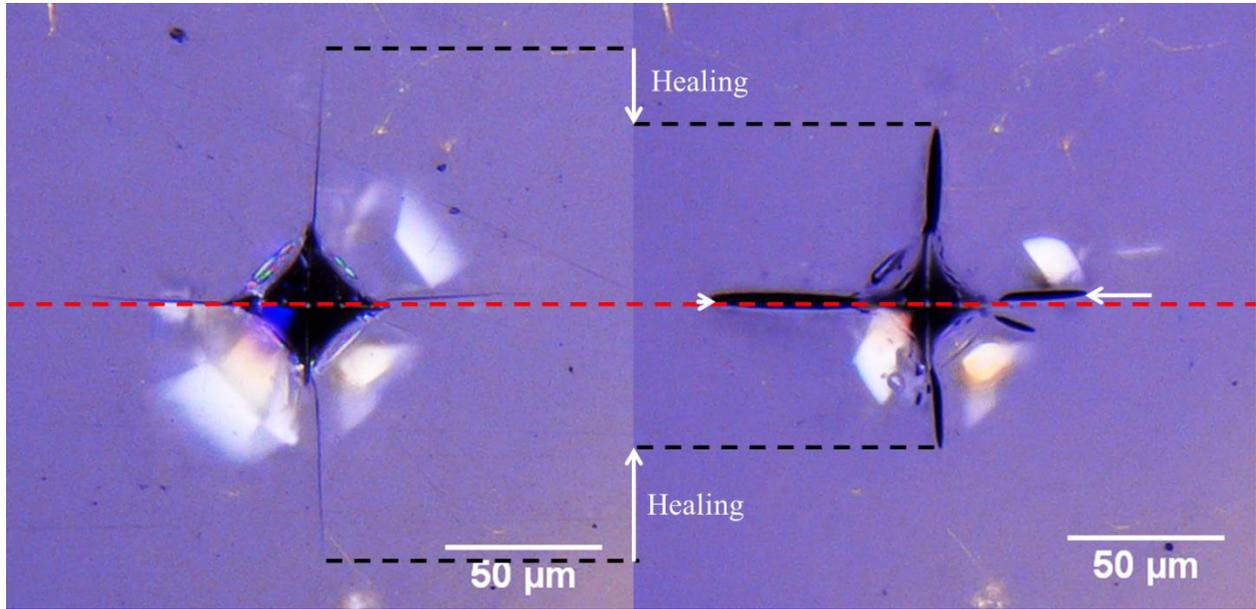
**Figure 4: Indent before (left) and after 10 min at 550°C (right). The red and black dashed lines represent guides for the eyes. The white arrows represent the decrease in crack length and by consequence the healing.**
