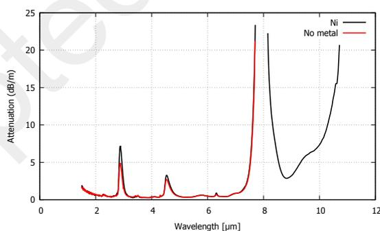
Fig. 4: Comparison between the attenuation spectra of a sample with Ni as a metal and a sample with no metal at all. In both samples TeCl<sub>4</sub> is used as hydrogen getter.
