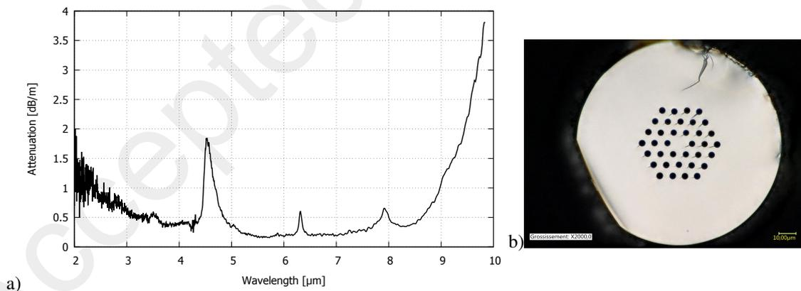
Fig. 3: Attenuation spectrum (a) and cross section (b) of a holey fiber obtained from the sample containing Mg and TeCl<sub>4</sub>.
