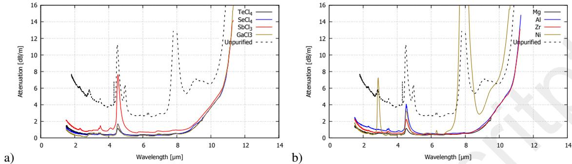
Fig. 2: Comparison between the attenuation spectra of Ge – As – Se fibers prepared using magnesium in combination with different hydrogen getters (a) and TeCl<sub>4</sub> in combination with different oxygen getters (b). In both graphs, an example of non purified glass is shown.
