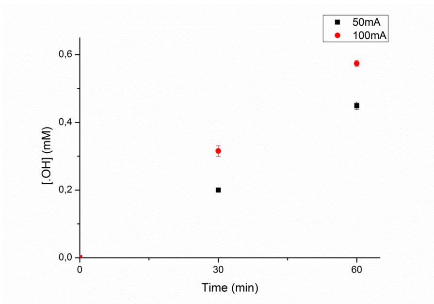
Figure 2. Concentration of generated  $\bullet\text{OH}$  as a function of the current density during 180 min of electrolysis, with DMSO 0.25M,  $40 \text{ mg}\cdot\text{L}^{-1} \text{ Fe}_3\text{O}_4$ , at pH 3, in 250 mL  $\text{Na}_2\text{SO}_4$  0.05M
