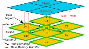
Fig. 3: Automated Multi-clusters Tiling with Fusion
