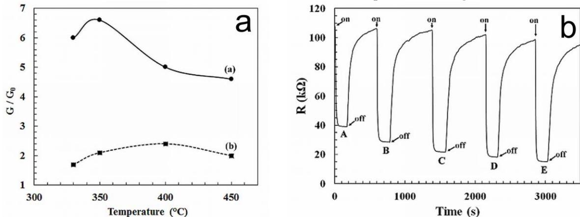
**Figure 3.** Sensitivity (fig. a) of the sensor-400 (plot a) and the sensor-500 (plot b) under 100 ppm of H<sub>2</sub>S in dry air as a function of the temperature. Dynamic response (fig. b) of the sensor-400 under A: 20 ppm, B: 40 ppm, C: 60 ppm, D: 80 ppm, E: 100 ppm of H<sub>2</sub>S at 350 °C. ON: H<sub>2</sub>S injected, OFF: air injected.
