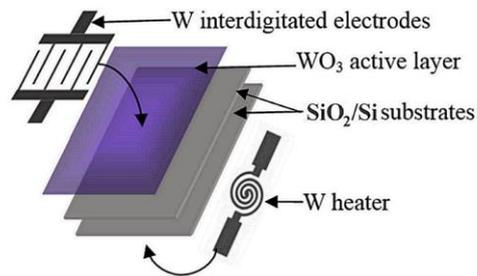
**Figure 1.** Structure of the gas sensor.
