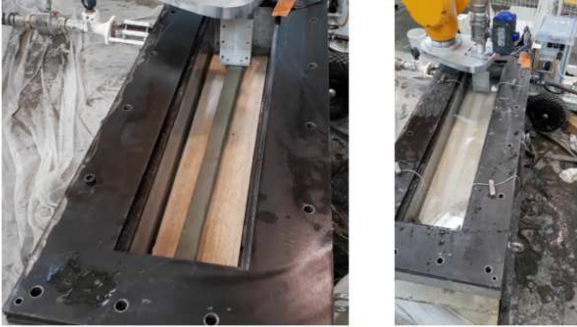
Fig. 2: Ongoing 3D printing of mortar –left: sample printed in air, right: sample printed in water.
