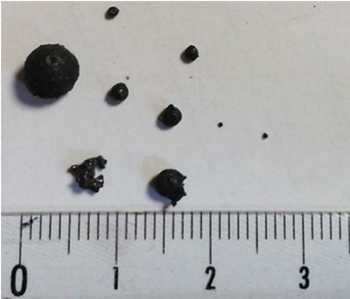
Figure 10: Metallic particles found in the char from Mix C – scale unit in cm
