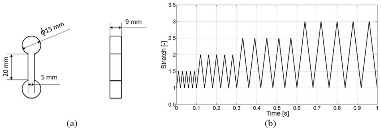
Fig. 10.1 (a) Sample geometry (b) loading conditions
