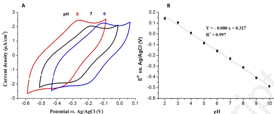
Figure 4: **A.** Cyclic voltammograms of 5ASA-based film onto glassy carbon electrode in 10 mM KCl solution at pH 8 (red), 7 (black) and 6 (blue). Scan rate: 5 mV/s. **B.** Influence of pH on the formal potential of the 5ASA-based film in commercial buffered solutions.
