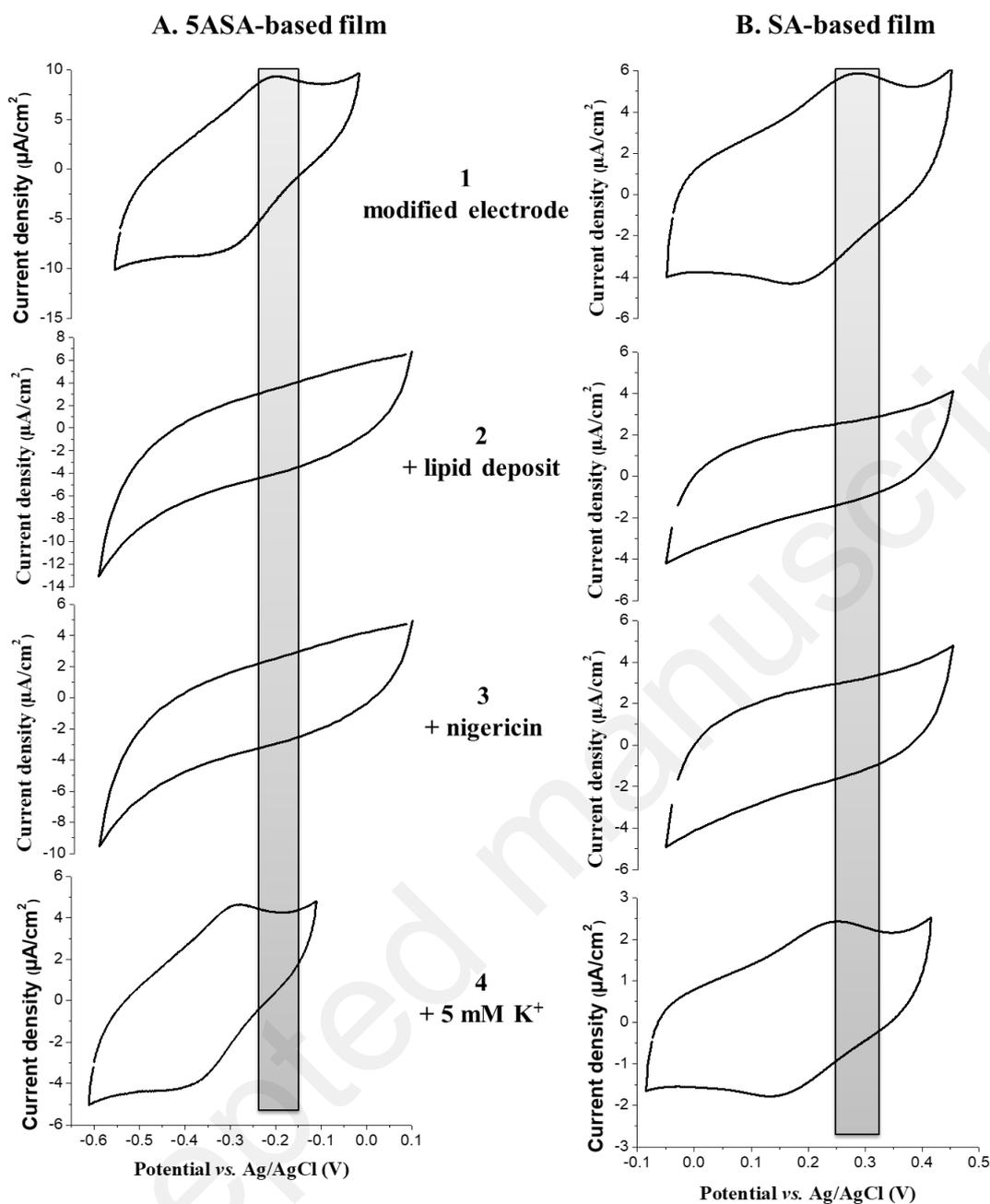
Figure 9: Experiments showing the study of (A) 5ASA- and (B) SA-modified electrodes (1) in 10 mM ammonium acetate at pH 7 at 100 mV/s under argon and room temperature (20°C). (2): After DMPC lipid deposition onto modified electrode. (3): After addition of nigericin in the supported DMPC lipid deposit onto the modified electrode. (4): After addition of 5 mM potassium acetate in solution. The grey stripes are indicative of the redox potentials and serve as a guide to the eye.
