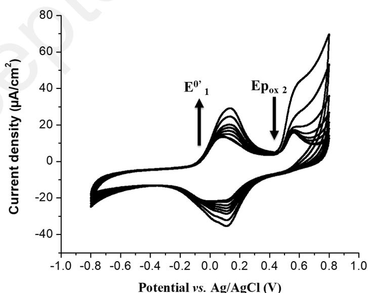
Figure 2: Consecutive cyclic voltammograms (8 scans) showing the electrodeposition of a
