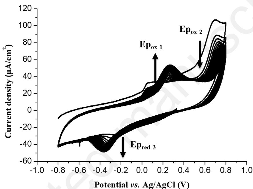
Figure 5: Consecutive cyclic voltammograms (20 scans) showing the formation of a SA-based redox active film from 1 mM SA in 10 mM phosphate buffer at pH 7 onto glassy carbon electrode. Scan rate: 100 mV/s.
