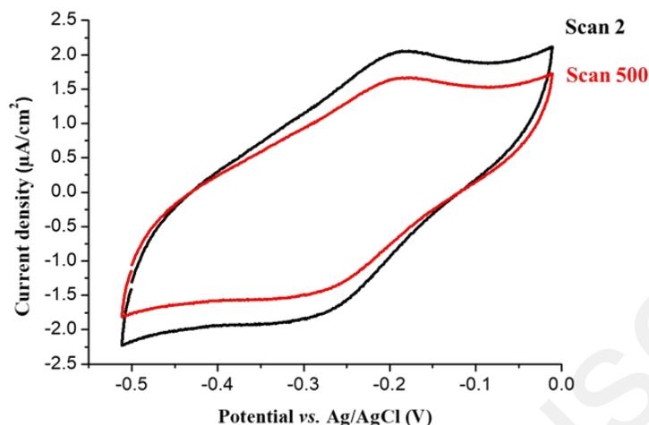
Figure 3: Cyclic voltammograms of 5ASA-based redox active film immobilized onto glassy carbon electrode after 2 (black) and 500 (red) consecutive scans in potassium phosphate buffer at pH 7. Scan rate: 5 mV/s.
