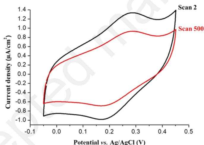
*Figure 6: Cyclic voltammograms of SA-based redox active film immobilized onto glassy carbon electrode after 2 (black) and 500 (red) consecutive scans recorded in ammonium acetate at pH 5. Scan rate: 5 mV/s.*
