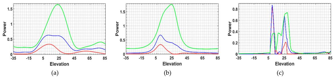
**Figure 7.** Extracted three-component features of forest pixel (shown in Figure 4a) from reconstructed T using (a) Beamforming, (b) Capon, (c) and the proposed method. Red, green and blue indicate the double-bounce, volumetric and surface scattering mechanisms.
