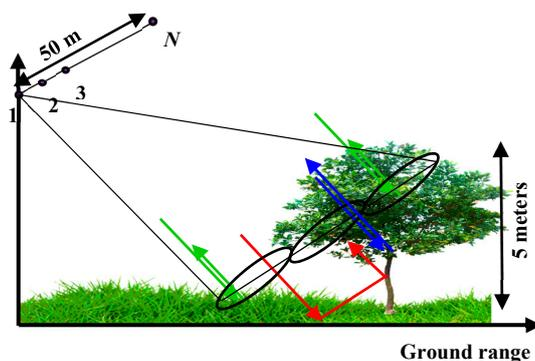
**Figure 1.** Simulated multi-baseline SAR geometry and the polarimetric backscatterings from forest. Red, green and blue indicate the double-bounce, volumetric and surface scattering mechanisms, respectively.
