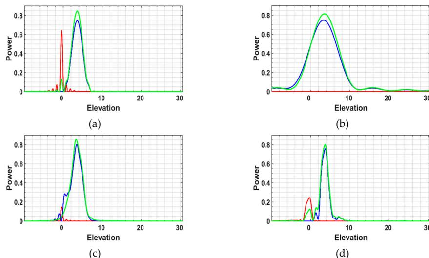
**Figure 3.** Extracted features from three-component decomposition of reconstructed  $\mathbf{T}$ . (a) simulated, (b) Beamforming, (c) Capon, and (d) proposed method. Red, green and blue indicate the profiles of double bounce, volumetric and surface scattering mechanisms.
