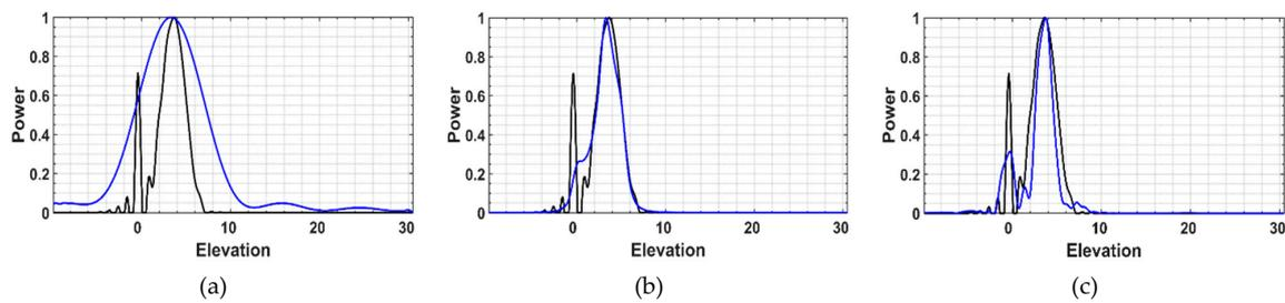
**Figure 2.** Extracted span profiles of the simulated scenario with full-rank reconstruction of  $\mathbf{T}$ , (a) Beamforming, (b) Capon, (c) the proposed method. Blue and black indicate the reconstructed and simulated signals.
