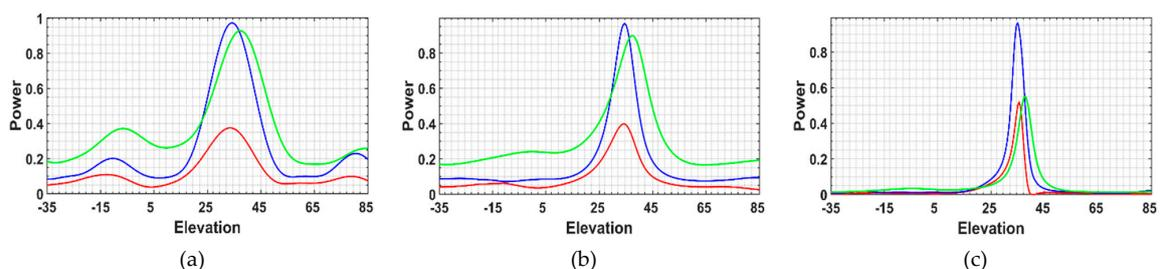
**Figure 6.** Extracted three-component features of ground pixel (shown in Figure 4a) from reconstructed  $T$  using (a) Beamforming, (b) Capon, and (c) the proposed method. Red, green and blue indicate the double-bounce, volumetric and surface scattering mechanisms.
